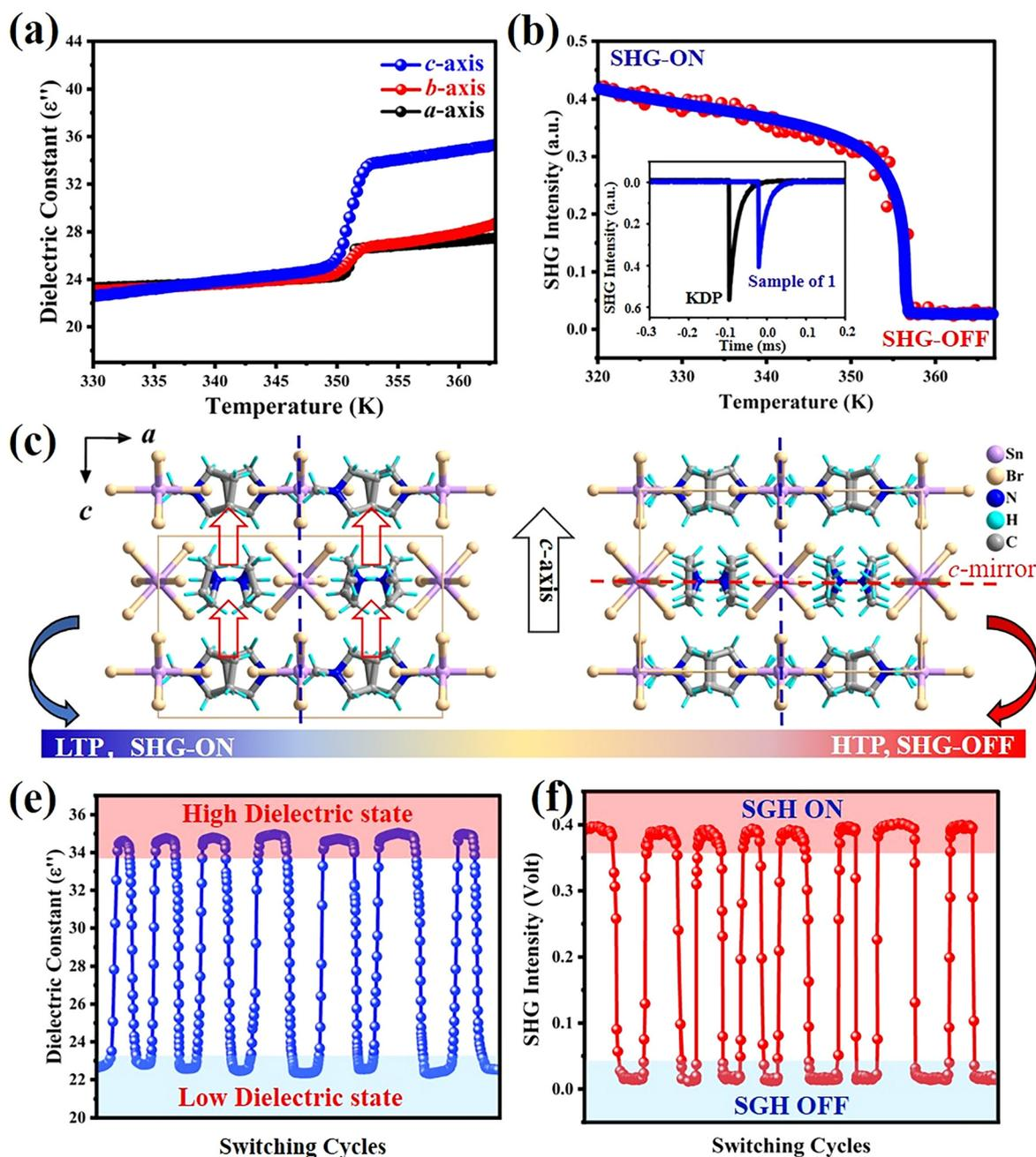
Fig. 6 (a) Variable-temperature dielectric constants of three crystallographic axes and (b) SHG signals. Inset: Oscilloscope traces of SHG signals of **1** compared with the reference KDP. (c) Schematic diagram of the appearance of symmetry breaking (e) switchable dielectric and (f) SHG properties after multiple heating-cooling cycles.
