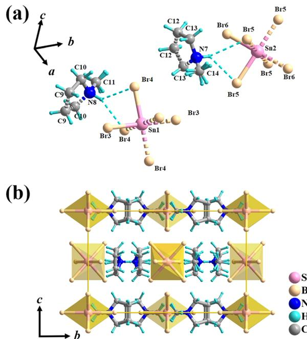
Fig. 2 (a) Asymmetric unit and (b) packing view of **1** along  $a$ -axis at 360 K. Dashed lines are used to link equivalent atoms generated by the symmetry operation except cyan dashed lines used to represent hydrogen bonds.
