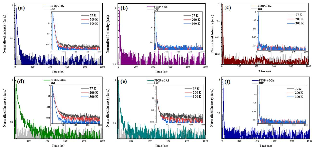
Fig. 4 Transient PL decays for these PhFIOP-based emitters doped in the mCP film (doping ratio: 10 wt %). The inset shows the temperature dependence of transient PL decay in degassed toluene. (a) **FIOP-o-Oz**, (b) **FIOP-o-Ad**, (c) **FIOP-o-Cz**, (d) **FIOP-o-2Oz**, (e) **FIOP-o-2Ad**, and (f) **FIOP-o-2Cz**. IRF: the instrument response functions of the light source.
