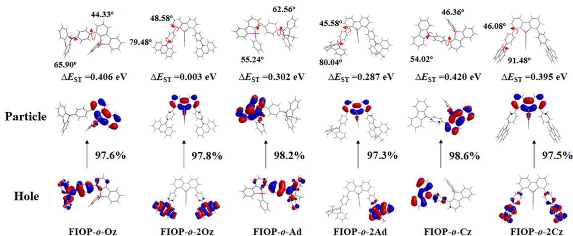
Fig. 5 NTO patterns (isocontour value = 0.030) for  $S_0 \rightarrow S_1$  excitations based on the optimized  $S_1$  geometries, together with the  $S_0$  geometry showing the twisting angle between the donor and the acceptor.
