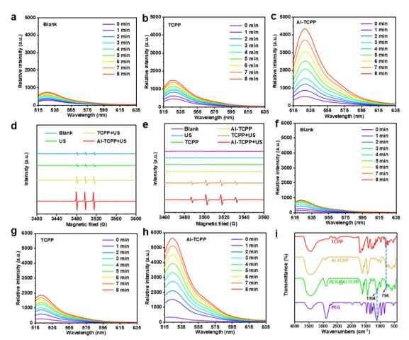
Fig. 3 The fluorescence spectra of (a-c) SOSG and (f-h) DCFH-DA in the presence of a blank sample, TCPP (50  $\mu$ g mL<sup>-1</sup>), and Al-TCPP (50  $\mu$ g mL<sup>-1</sup>) under US (50 kHz, 1.6 W cm<sup>-2</sup>, 8 min) irradiation. (d) The TEMP/ $^{1}$ O<sub>2</sub> ESR spectra of a blank sample, US, TCPP + US, and Al-TCPP + US. (e) The DMPO/·OH ESR spectra of a blank sample, US, TCPP + US, and Al-TCPP + US. (i) FT-IR spectra of TCPP, Al-TCPP, PEG@Al-TCPP, and PEG
