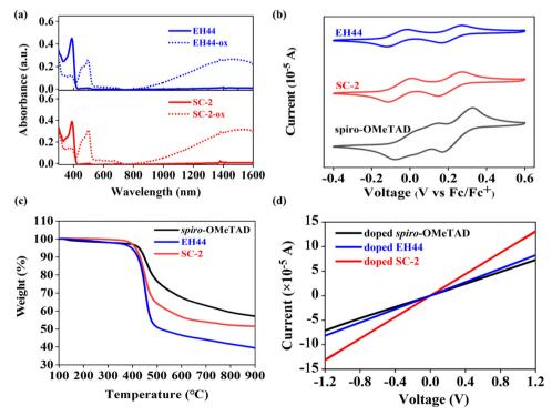
Fig. 2 (a) UV-Vis absorption spectra of EH44, EH44-ox and SC-2, SC-ox in chloroform. (b) CV of pristine spiro-OMeTAD, EH44, and pristine SC-2. (c) TGA curves of spiro-OMeTAD, EH44, and SC-2. (d) I-V curves of doped spiro-OMeTAD, doped EH44, and doped SC-2 films.
