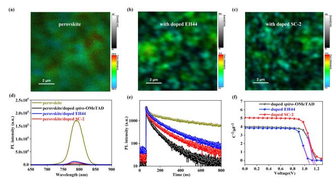
Fig. 5 FLIM images of the (a) perovskite and perovskite covered with (b) doped EH44, and (c) doped SC-2. (d) Steady-state PL spectra, and (e) TRPL spectra of the perovskite w/o HTL covering. The sample structure is glass|perovskite|HTL. (f) Mott-Schottky plots of solar cells.
