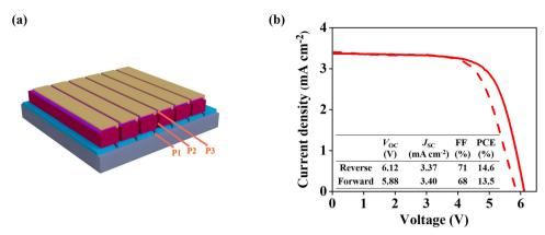
Fig. 7 (a) Schematic diagram of a FTO|SnO<sub>2</sub>|perovskite|HTL|Au perovskite solar module (full size: 5 cm × 5 cm, with 6 series-connected sub-cells). (b) J-V curve of the best-performing module under AM 1.5G 1 sun irradiation based on spin-coated perovskite and doped SC-2 HTL with a mask area of 10.0 cm<sup>2</sup>.
