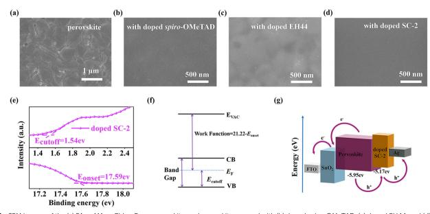
Fig. 3 SEM images of the (a)  $FA_{0.92}MA_{0.08}PbI_{2.76}Br_{0.24}$  perovskite, and perovskite covered with (b) doped spiro-OMeTAD, (c) doped EH44, and (d) doped SC-2. (e) UPS of the doped SC-2 film. (f) Energy band diagram of the doped SC-2 film in UPS measurement. (g) Schematic illustration of the energy level diagram of each layer in PSCs. The sample structure in SEM and UPS measurement is  $FTO[SnO_2|FA_{0.92}MA_{0.08}PbI_{2.76}Br_{0.24}]$  HTL.
