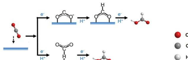
Fig. 7 Schematic diagram of the  $2\text{e}^-$  reaction path in  $\text{eCO}_2\text{RR}$ . Copyright 2021, Elsevier.<sup>65</sup>
