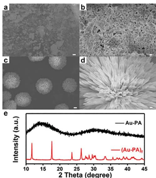
Fig. 5 SEM images of Au-PA precursors at (a) 5  $\mu\text{m}$ , (b) 500 nm and (Au-PA)<sub>f</sub> precursors at (c) 5  $\mu\text{m}$ , (d) 500 nm. (e) XRD patterns of the amorphous Au-PA precursor generated without ethanol and the flower-like (Au-PA)<sub>f</sub> precursor generated with the presence of ethanol. Copyright 2020, Royal Society of Chemistry.<sup>54</sup>
