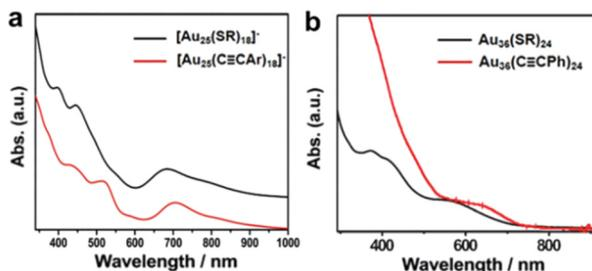
Fig. 3 The comparison of optical properties of (a)  $[\text{Au}_{25}(\text{PhC}\equiv\text{C}\text{Ar})_{18}]^-$ ,  $[\text{Au}_{25}(\text{SR})_{18}]^-$  and (b)  $\text{Au}_{36}(\text{PhC}\equiv\text{C})_{24}$ ,  $\text{Au}_{36}(\text{SR})_{24}$ . Copyright 2017 and 2018, Wiley.<sup>38,39</sup>
