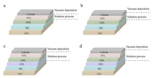
Fig. 6 Basic device structures and processing method of solution-processed OLEDs with (a) solution-processed HIL/EML, (b) solution-processed HIL/EML EML/ETL, (c) HIL/HTL/EML, and (d) HIL/HTL/EML/ETL, respectively
