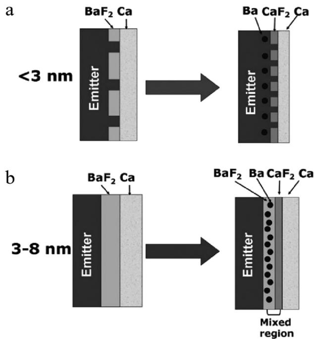
Fig. 7 Schematic diagrams of the contact between the cathode ( $\text{BaF}_2/\text{Ca}/\text{Al}$ ) and the emitter for (a) a thin  $\text{BaF}_2$  layer with a thickness less than 3 nm, and (b) a  $\text{BaF}_2$  layer with a thickness of 3–8 nm.<sup>155</sup> Copyright 2009 Wiley-VCH Verlag GmbH & Co. KGaA, Weinheim.
