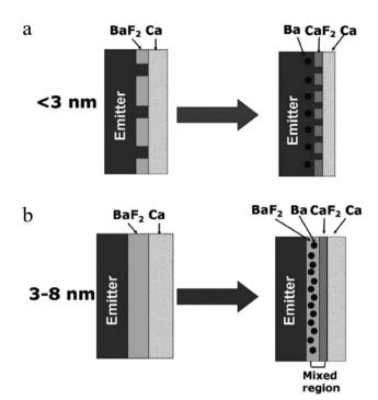
Fig. 7 Schematic diagrams of the contact between the cathode (BaF<sub>2</sub>/Ca/ Al) and the emitter for (a) a thin BaF<sub>2</sub> layer with a thickness less than 3 nm, and (b) a  $BaF_2$  layer with a thickness of 3–8 nm. <sup>155</sup> Copyright 2009 Wiley-VCH Verlag GmbH & Co. KGaA, Weinheim.
