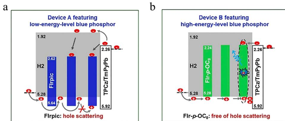
Fig. 8 Effect analysis of hole scattering. (a) Working mechanism of the  $\text{FIRpic}$ -based blue device. (b) Working mechanism of the  $\text{FIR-p-OC}_8$ -based blue device.<sup>160</sup> Copyright 2018 Elsevier.
