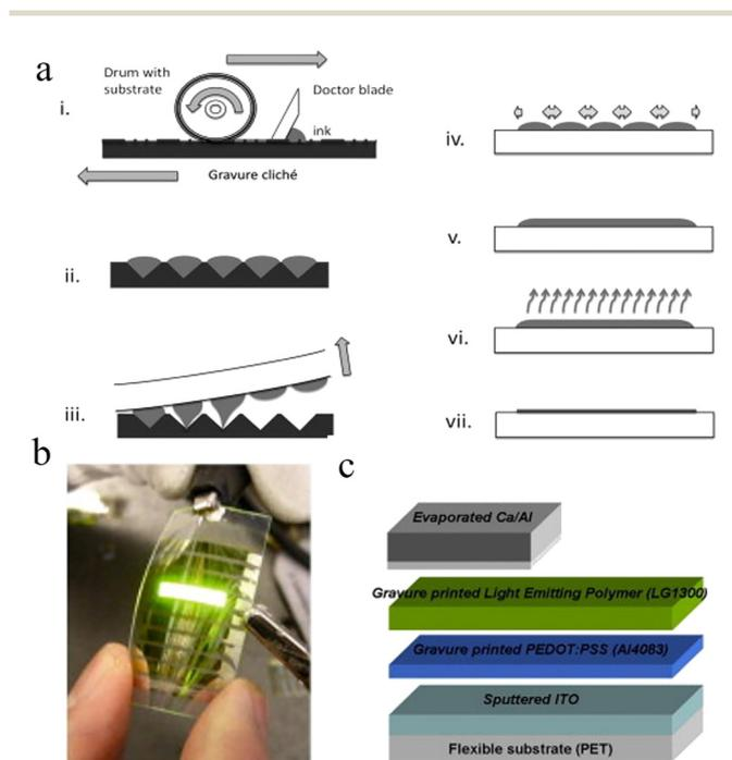
Fig. 14 (a) Gravure printing process. (b) Photograph of light emission from a fully printed flexible PLED of fully gravure printed and fully spin-coated PLEDs. The size of the light emission area is  $0.42 \text{ cm}^2$  (width:  $1.4 \text{ cm}$ , height:  $0.3 \text{ cm}$ ). (c) Structure of gravure printed PLEDs.<sup>192</sup> Copyright 2010 Elsevier B.V.
