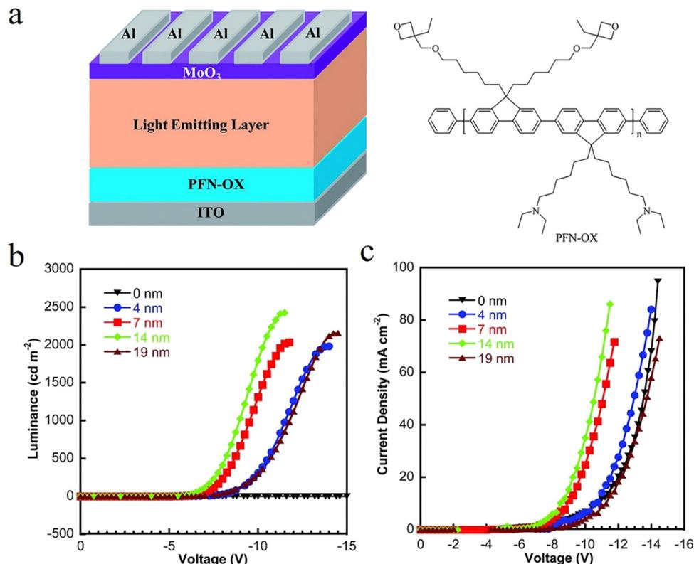
Fig. 3 (a) The device configuration of the inverted OLED and the chemical structures of PFN-OX and light emitting layer materials used in this study. (b)  $L$ - $V$  and (c)  $J$ - $V$  curves of blue light devices with different thicknesses of the PFN-OX interlayer.<sup>91</sup> Copyright 2014 The Royal Society of Chemistry.
