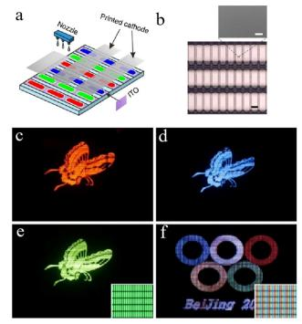
Fig. 9 Device structures and photographs of monochrome and full-color displays. (a) Schematic of the full color structure. (b) Microscopic image of the back of the display. (c) Red, (d) blue and (e) green monochrome displays. (f) Full-color display with a microscopic image. 166 Copyright 2013, Nature Publishing Group.
