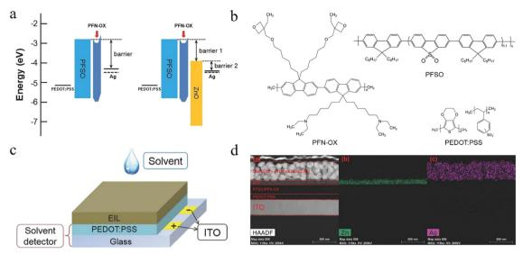
Fig. 4 (a) Energy level diagrams of the device. (b) Chemical structures of PFSO, PFN-OX, and PEDOT:PSS. (c) Schematic illustration of the "solvent detector." (d) EDS map of the all-solution-processed OLED. 101 Copyright 2018 Wiley-VCH Verlag GmbH & Co. KGaA, Weinheim.
