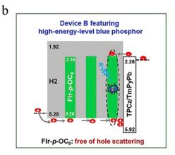
Fig. 8 Effect analysis of hole scattering. (a) Working mechanism of the FIrpic-based blue device. (b) Working mechanism of the FIrp-OC<sub>8</sub>-based blue device. 160 Copyright 2018 Elsevier.
