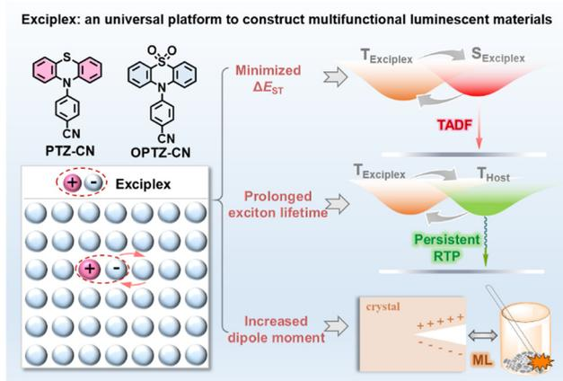
Fig. 1 Exciplex-induced thermally-activated delayed fluorescence (TADF), persistent room temperature phosphorescence (RTP) and mechanoluminescence (ML) in a doping system with **OPTZ-CN** as the host and **PTZ-CN** as the guest.
