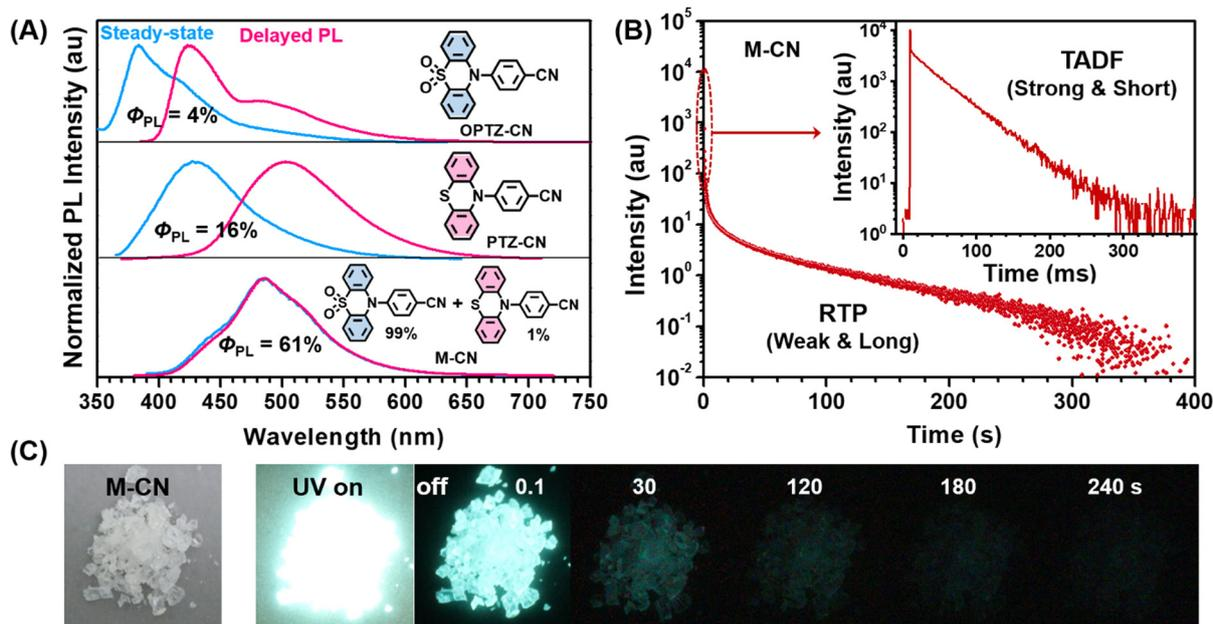
Fig. 2 (A) The steady-state and delayed photoluminescence (PL) spectra of the **OPTZ-CN** crystal, **PTZ-CN** crystal and corresponding host-guest doping system (**M-CN**); (B) the PL decay curves of **M-CN**; (C) the luminescent behavior of **M-CN** ( $\lambda_{ex} = 365$  nm).
