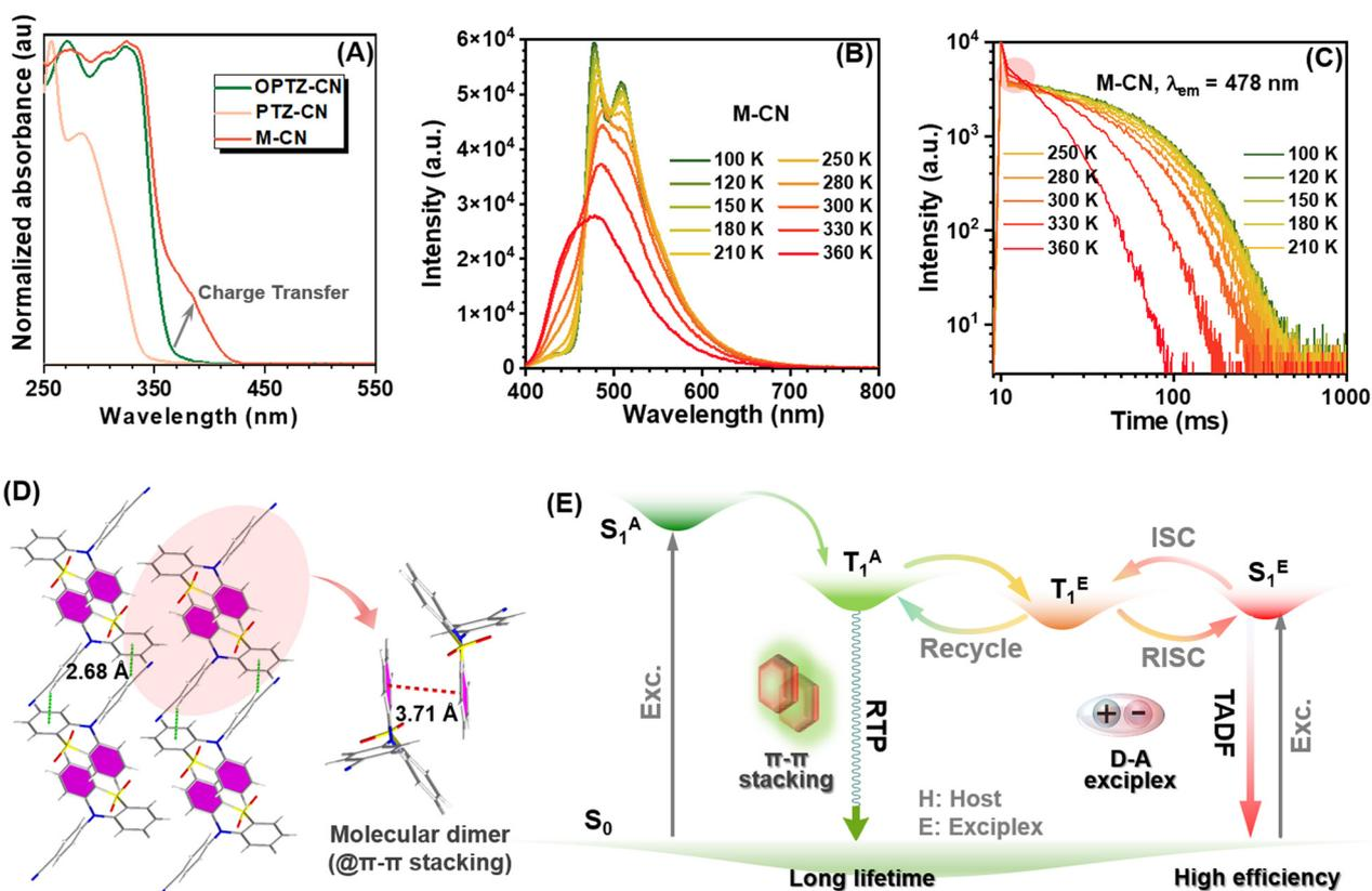
Fig. 3 (A) Normalized UV-Vis absorption spectra of the **OPTZ-CN** crystal, **PTZ-CN** solution and **M-CN** crystal; (B) temperature-dependent PL spectra of the **M-CN** crystal; (C) temperature-dependent PL decay curves of the **M-CN** crystal at 478 nm; (D) single crystal structure of the **OPTZ-CN** crystal; (E) proposed mechanism for the unique luminescent behaviors of the **M-CN** crystal.
