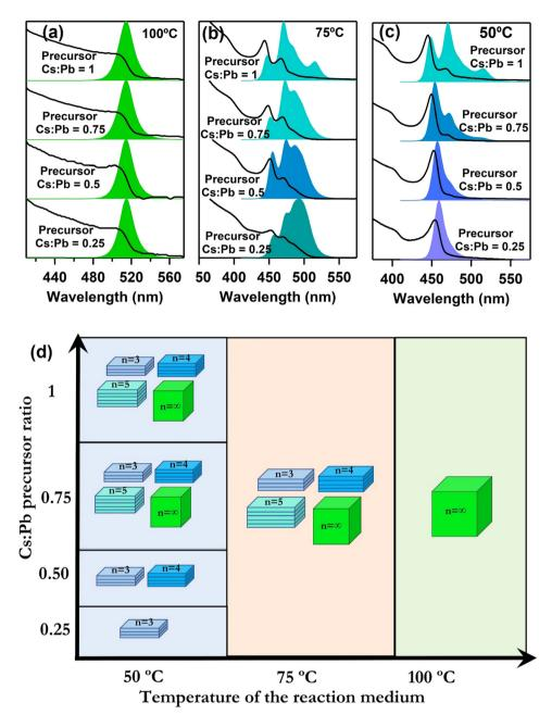
Fig. 4 Effect of cesium to lead precursor (Cs:Pb) ratio (1 to 0.25 from top to bottom) on absorption and PL properties of CsPbBr<sub>3</sub> NCs synthesized in a LAMe DES medium (CPB-LAMe) for three different reaction temperatures (a)100 °C (b) 75 °C (c) 50 °C. (d) Schematic representation for the formation of CsPbBr<sub>3</sub> NPLs/NC having different thicknesses as a function of temperature and cesium to lead precursor ratio.
