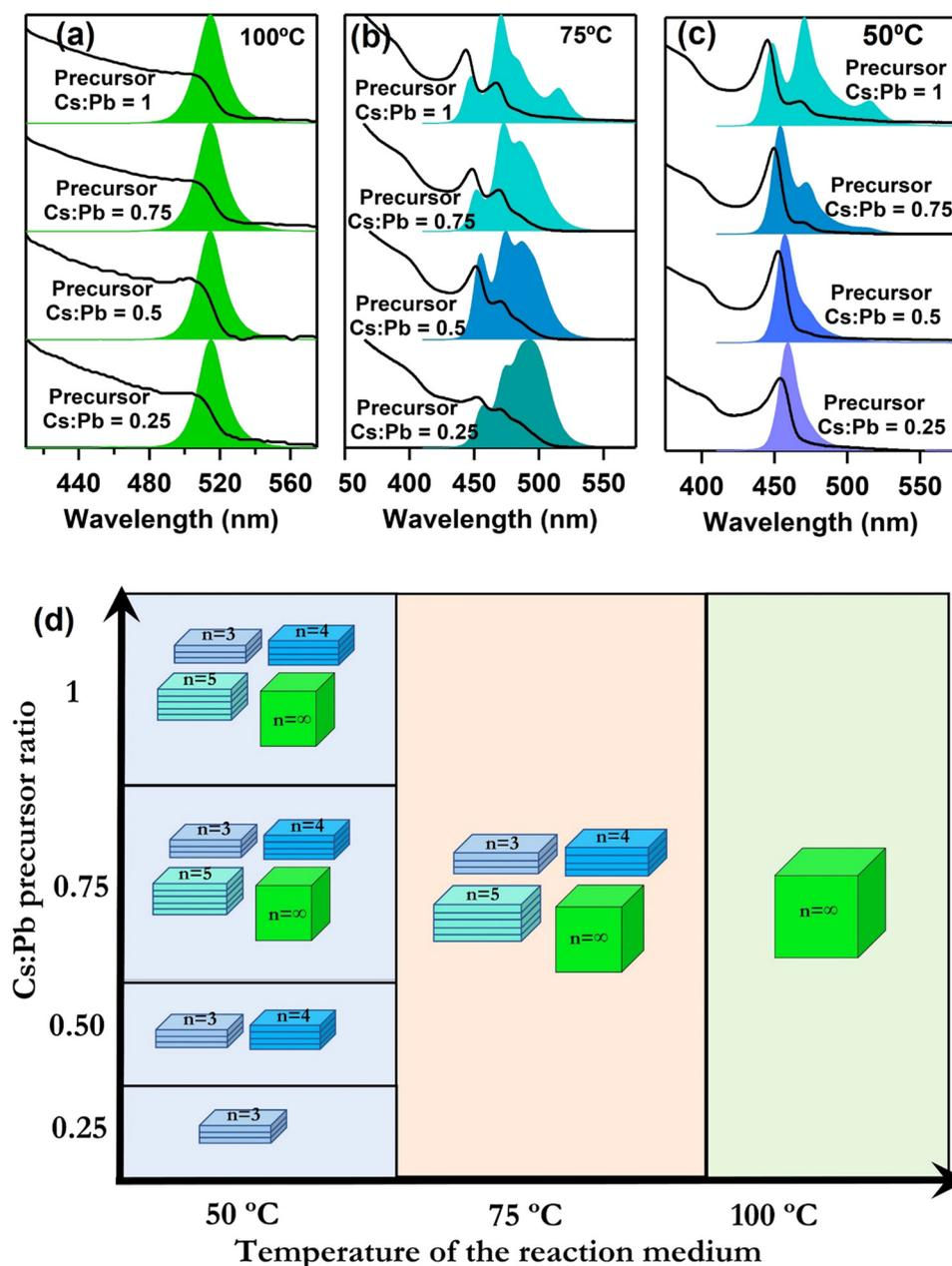
Fig. 4 Effect of cesium to lead precursor (Cs:Pb) ratio (1 to 0.25 from top to bottom) on absorption and PL properties of CsPbBr<sub>3</sub> NCs synthesized in a LAME DES medium (CPB-LAME) for three different reaction temperatures (a) 100 °C (b) 75 °C (c) 50 °C. (d) Schematic representation for the formation of CsPbBr<sub>3</sub> NPLs/NC having different thicknesses as a function of temperature and cesium to lead precursor ratio.
