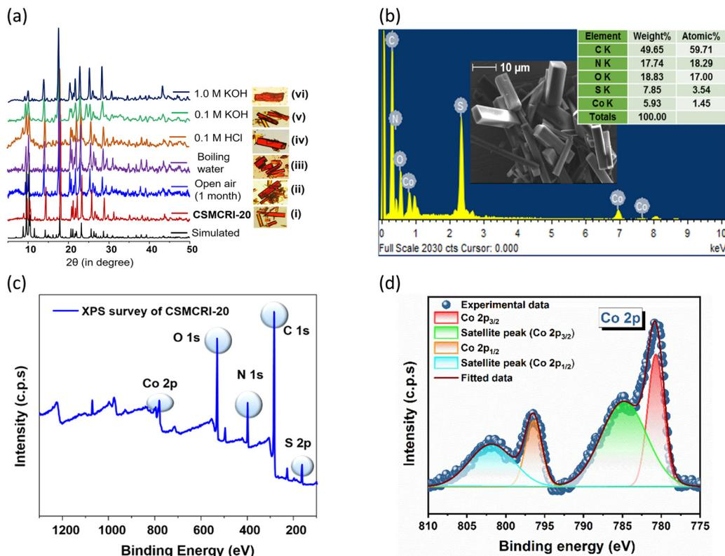
Fig. 2 (a) PXRD patterns and optical images of the MOF under different experimental conditions, (i) as made **CSMCRI-20**, under (ii) open air (1 month), (iii) boiling water, (iv) 0.1 M HCl, (v) 0.1 M KOH and (vi) 1 M KOH. (b) FE-SEM image and EDX analysis of **CSMCRI-20**. (c) XPS survey spectra of the framework. (d) High-resolution XPS spectrum of Co 2p.
