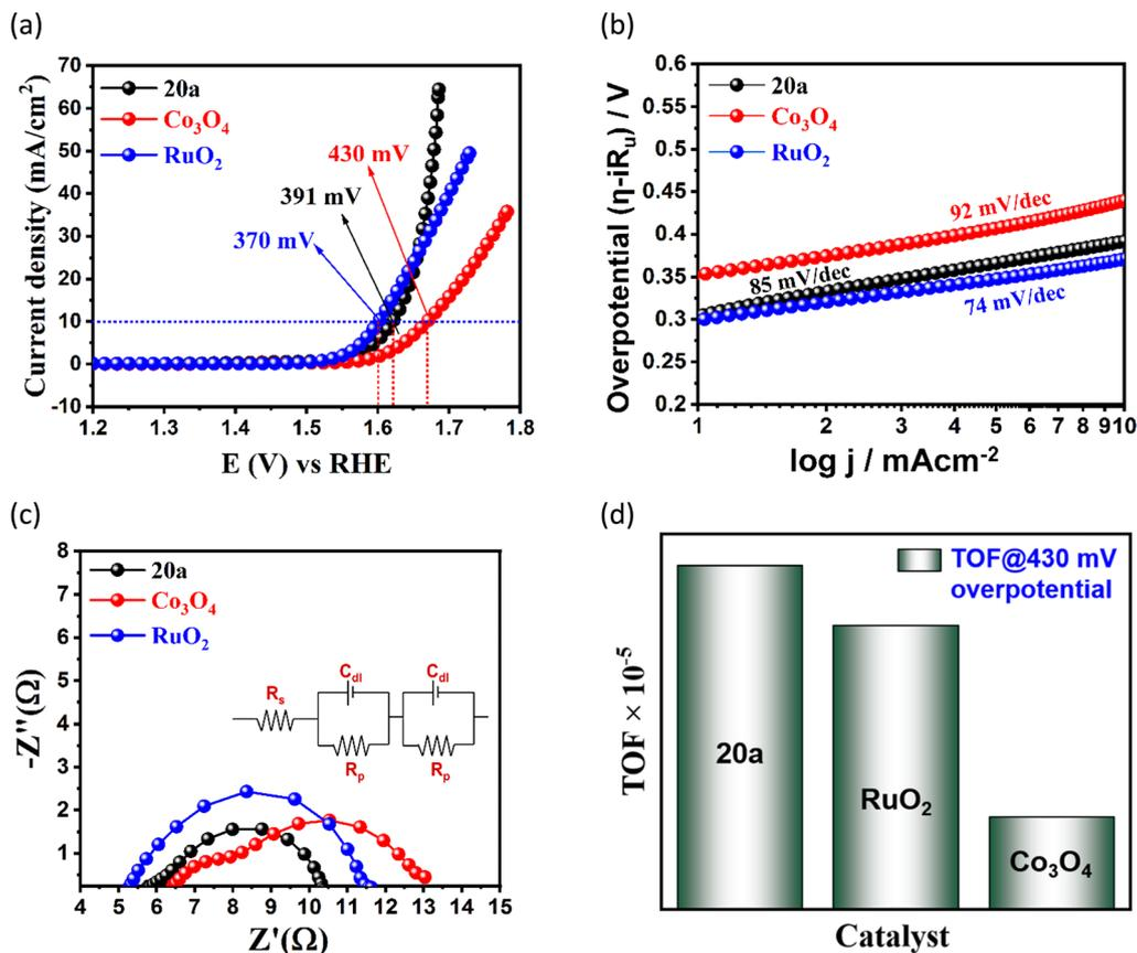
Fig. 3 (a) Linear sweep voltammetry (LSV) for the present MOF and other benchmark commercial electrocatalysts. (b) Tafel plot for activated CSMCRI-20. (c) Electrochemical impedance spectra (EIS) of **20a** at  $10 \text{ mA cm}^{-2}$ . (d) Turn-over frequency (TOF) values for **20a**,  $\text{RuO}_2$  and  $\text{Co}_3\text{O}_4$ .
