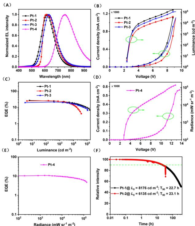
Fig. 4 (A) Normalized EL spectra of the selected red and NIR devices doped with **Pt-1** (6 wt%), **Pt-2** (9 wt%), **Pt-3** (6 wt%) and **Pt-4** (3 wt%). (B)  $J$ – $V$ – $L$  characteristics and (C) EQE versus the luminance of the red OLEDs doped with **Pt-1** (6 wt%), **Pt-2** (9 wt%) and **Pt-3** (6 wt%). (D)  $J$ – $V$ – $R$  characteristics and (E) EQE versus the radiance of the NIR OLEDs doped with **Pt-4** (3 wt%). (F) Normalized current density of the device versus operating time.
