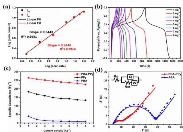
Fig. 5 (a) The plot of the logarithm of peak current vs. the logarithm of scan rate; (b) galvanostatic charge-discharge curves of Co-Co@Ni-Fe PBA-PPy composite at different current densities; (c) comparing the specific capacitance of all materials at increasing current densities; and (d) Nyquist plots of Co-Co@Ni-Fe PBA-PPy and Co-Co@Ni-Fe core-shell PBA composites at a fully charged state.
