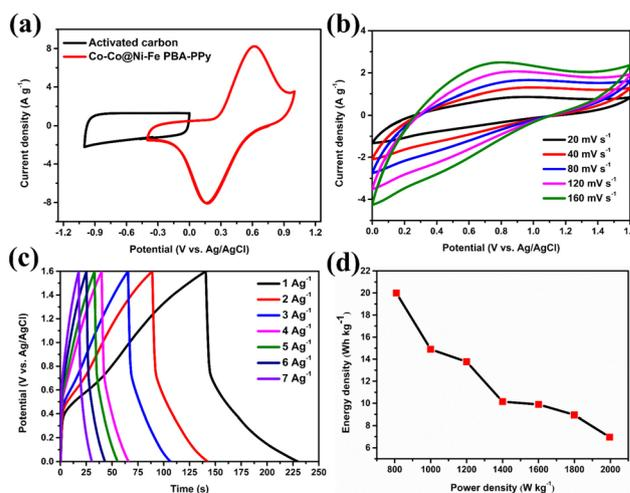
Fig. 6 (a) CV curves of AC and Co-Co@Ni-Fe PBA-PPy composite at 40 mV s<sup>-1</sup> in 1.0 M Na<sub>2</sub>SO<sub>4</sub>. (b) CV curves, (c) GCD curves, and (d) Ragone plot of the Co-Co@Ni-Fe PBA-PPy//AC device.
