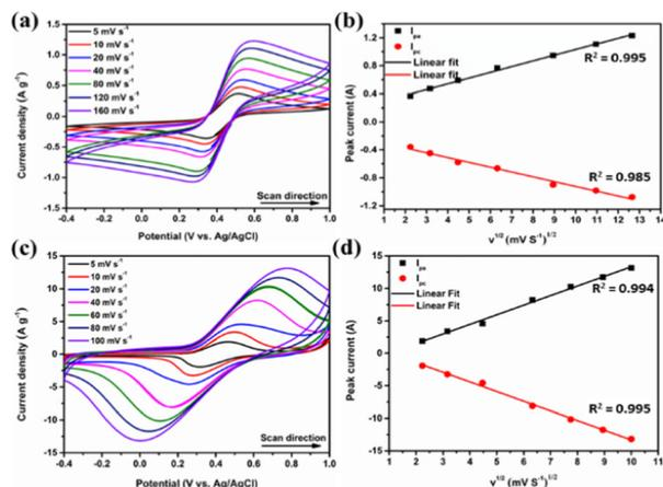
Fig. 4 (a) CV curves of Co-Co@Ni-Fe core-shell PBA at different scan rates in 1.0 M Na<sub>2</sub>SO<sub>4</sub>; (b) the dependency of the peak currents on the square root of scan rates; (c) CV profiles of the Co-Co@Ni-Fe PBA-PPy composite at various scan rates in 1.0 M Na<sub>2</sub>SO<sub>4</sub>; (d) the plot of peak currents against the square root of scan rates.
