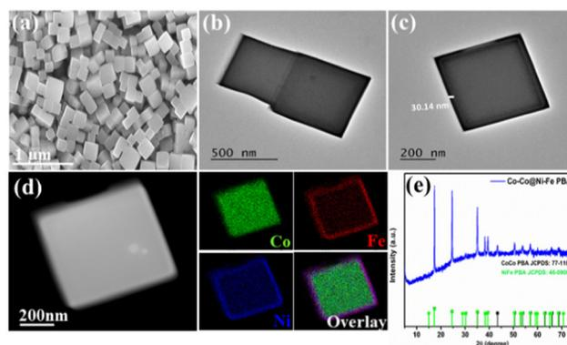
**Fig. 1** (a) HR-SEM image; (b), (c) TEM images; (d) STEM image of core-shell PBA and the corresponding elemental mapping of the same frame showing Co, Fe, and Ni with their overlay; (e) XRD patterns of Co-Co@Ni-Fe core-shell PBA.
