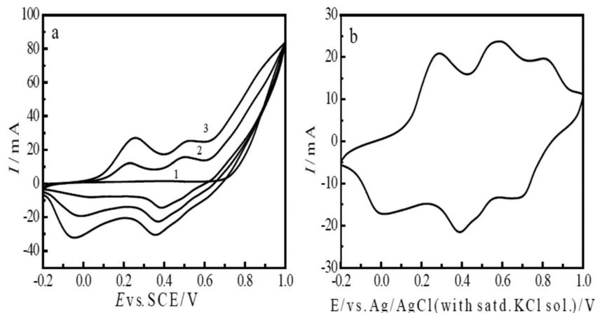
Fig. 1 (a) CVs of the electrochemical synthesis of the polyaniline film on graphite obtained in a solution containing 0.2 M aniline and 0.6 M H<sub>2</sub>SO<sub>4</sub>; (b) the CV of the polyaniline film in a 0.2 M H<sub>2</sub>SO<sub>4</sub> solution at a scan rate of 60 mV s<sup>-1</sup>.
