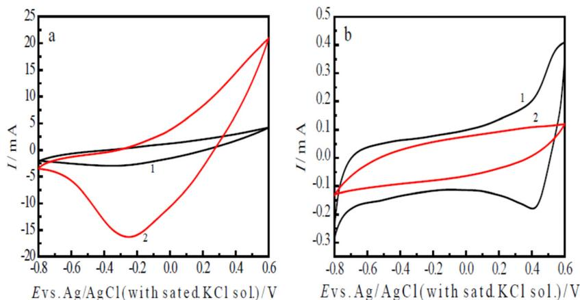
Fig. 4 The CVs of different types of electrodes at a scan rate of 60 mV s<sup>-1</sup>. (a) Curve 1: nano-PAN/N-graphite electrode in CO<sub>2</sub>-saturated water and curve 2: nano-PAN/T-graphite electrode in CO<sub>2</sub>-saturated water; (b) curve 1: nano-PAN/T-graphite electrode in a H<sub>2</sub>SO<sub>4</sub> solution of pH 3.8 and curve 2: nano-T-graphite electrode in CO<sub>2</sub>-saturated water.
