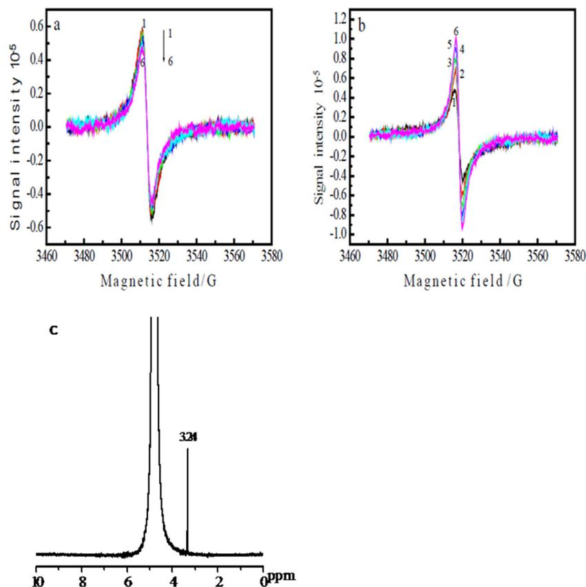
Fig. 6 The ESR spectra of the PAN/Pt electrodes at various potentials (a) in a  $\text{H}_2\text{SO}_4$  solution of pH 3.8; (b) in  $\text{CO}_2$ -saturated water free of the supporting electrolyte of pH 3.8 at different potentials: (1)  $-0.2$ , (2)  $-0.4$ , (3)  $-0.6$ , (4)  $-0.8$ , (5)  $-1.0$ , and (6)  $-1.2 \text{ V}$  (vs. Ag/AgCl with a saturated KCl solution); (c) the  $^1\text{H}$  NMR spectrum of the product solution.
