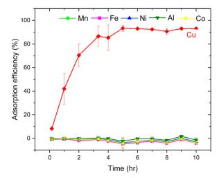
Adsorption efficiency of metal ions over the period of time.
