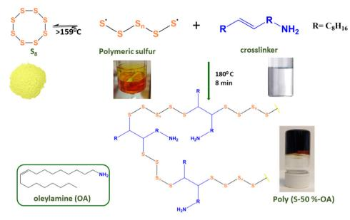
Scheme 1 Schematic illustration for the synthesis of poly(S-50%-OA). The structure of the crosslinker (oleylamine) is shown in the inset.
