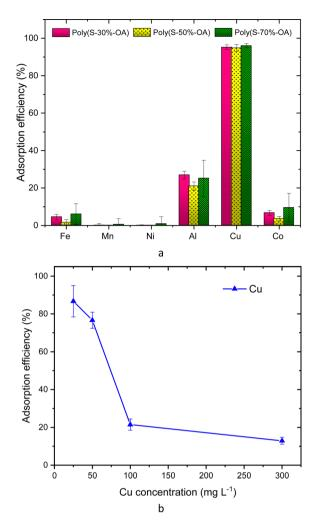
Fig. 7 Adsorption efficiency of metal ions with varying (a) sulfur content in poly(S-r-OA) (r = 30, 50, 70 wt%) (b) Cu concentration (mg L<sup>-1</sup>) in solution using 0.5 g poly(S-50%-OA) adsorbent.
