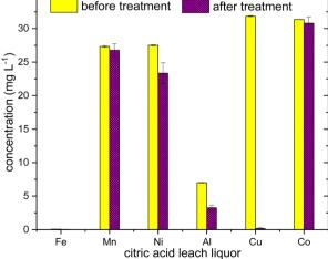
Fig. 10 Metal selectivity profile of poly(S-50%-OA) treated in HCl and citric acid leach liquor in terms of concentration (mg  $L^{-1}$ ) before and after adsorption. Initial concentration of  $Cu^{2+}$  ion was diluted to 30 mg  $L^{-1}$ .
