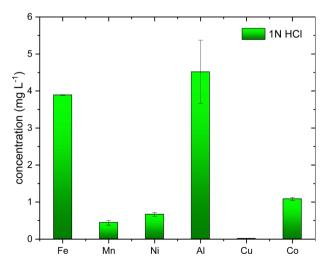
Fig. 9 Desorption/regeneration of metal ions after treating poly(S-50%-OA) recovered after adsorption in 1 N HCl for 6 h.
