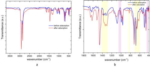
Fig. 4 ATR-FTIR spectra of poly(S-50%-OA) before and after adsorption (a) 3700-400 cm<sup>-1</sup> (full spectra) (b) zoom spectra in the fingerprint region.
