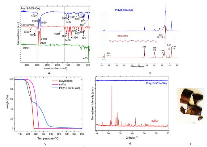
Fig. 1 Characterization of poly(S-50%-OA) (a) AT-FTIR (b) <sup>1</sup>H-NMR (c) TGA (d) PXRD (e) photograph of the material.
