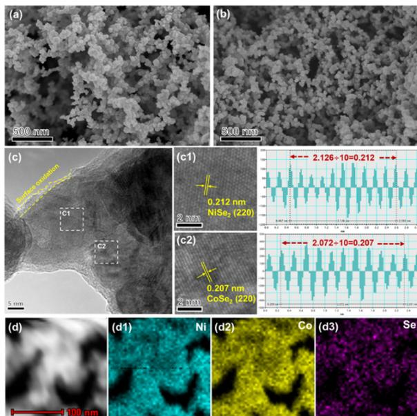
Fig. 2 (a and b) SEM images of the Ni-Co and NiSe<sub>2</sub>-CoSe<sub>2</sub> aerogel. (c) HRTEM image of the NiSe<sub>2</sub>-CoSe<sub>2</sub> aerogel with lattice fringes of NiSe<sub>2</sub> and CoSe<sub>2</sub> (c1 and c2). (d) STEM image of the NiSe<sub>2</sub>-CoSe<sub>2</sub> aerogel and its corresponding EDX mapping of Ni, Co, Se (d1–d3).
