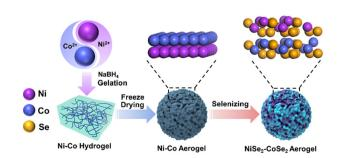
Fig. 1 Schematic illustration of the synthesis of Ni-Co and NiSe<sub>2</sub>-CoSe<sub>2</sub> aerogels.
