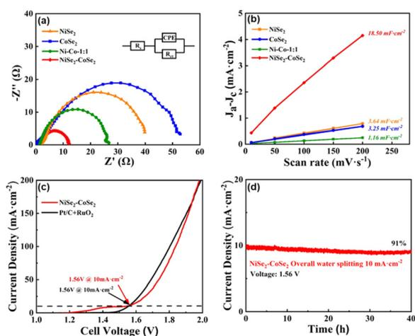
Fig. 6 (a) EIS measurements of prepared samples. (b)  $C_{dl}$  values of prepared samples. (c) LSV measurements for overall water splitting performance of the devices based on NiSe<sub>2</sub>-CoSe<sub>2</sub> electrodes and Pt/C + RuO<sub>2</sub> electrodes. (d) Chronoamperometric measurement of NiSe<sub>2</sub>-CoSe<sub>2</sub> aerogel toward overall water splitting.
