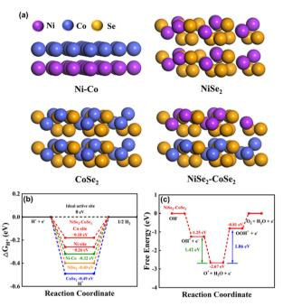
Fig. 7 (a) Crystal models of Ni-Co, NiSe2, CoSe2, and NiSe2-CoSe2 constructed based on the XRD. (b) Free energy diagram of the HER for different catalysts. (c) Free energy diagram of the OER for NiSe2-CoSe2.
