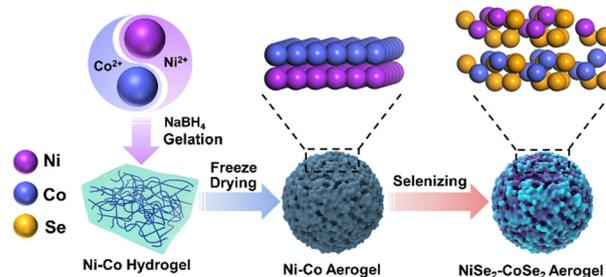
Fig. 1 Schematic illustration of the synthesis of Ni–Co and NiSe<sub>2</sub>–CoSe<sub>2</sub> aerogels.
