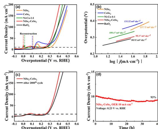
Fig. 5 (a and b) Polarization LSV curves and Tafel slopes of NiSe<sub>2</sub>-CoSe<sub>2</sub>, NiSe<sub>2</sub> and CoSe<sub>2</sub> aerogels and RuO<sub>2</sub> toward the OER in 1.0 M KOH. (c) Cyclic stability of NiSe<sub>2</sub>-CoSe<sub>2</sub> toward the OER. (d) Chronoamperometric measurement of NiSe<sub>2</sub>-CoSe<sub>2</sub> toward the OER.
