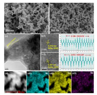
Fig. 2 (a and b) SEM images of the Ni-Co and NiSe2-CoSe2 aerogel. (c) HRTEM image of the NiSe<sub>2</sub>-CoSe<sub>2</sub> aerogel with lattice fringes of NiSe<sub>2</sub> and CoSe<sub>2</sub> (c1 and c2). (d) STEM image of the NiSe<sub>2</sub>-CoSe<sub>2</sub> aerogel and its corresponding EDX mapping of Ni, Co, Se (d1-d3).
