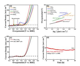
Fig. 5 (a and b) Polarization LSV curves and Tafel slopes of NiSe<sub>2</sub>-CoSe<sub>2</sub>, NiSe<sub>2</sub> and CoSe<sub>2</sub> aerogels and RuO<sub>2</sub> toward the OER in 1.0 M KOH. (c) Cyclic stability of NiSe2-CoSe2 toward the OER. (d) Chronoamperometric measurement of NiSe2-CoSe2 toward the OER
