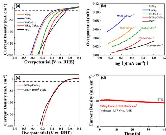
Fig. 4 (a and b) Polarization LSV curves and Tafel slopes of NiSe<sub>2</sub>, CoSe<sub>2</sub>, Ni-Co, and NiSe<sub>2</sub>-CoSe<sub>2</sub> aerogels and Pt/C toward the HER in 1.0 M KOH. (c) Cyclic stability of NiSe<sub>2</sub>-CoSe<sub>2</sub> toward the HER. (d) Chronoamperometric measurement of NiSe<sub>2</sub>-CoSe<sub>2</sub> toward the HER.
