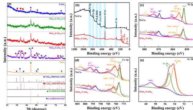
Fig. 3 (a) XRD patterns of the NiSe<sub>2</sub>-CoSe<sub>2</sub> aerogel and comparison samples. (b) XPS survey spectrum of Ni-Co and NiSe<sub>2</sub>-CoSe<sub>2</sub> aerogels. (c and d) High resolution Ni 2p and Co 2p XPS spectra of Ni-Co and NiSe<sub>2</sub>-CoSe<sub>2</sub> aerogels. (e) High resolution Se 3d XPS spectra of the NiSe<sub>2</sub>-CoSe<sub>2</sub> aerogel.
