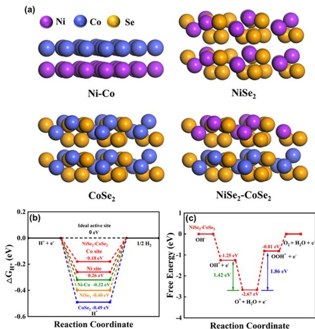
Fig. 7 (a) Crystal models of Ni-Co, NiSe<sub>2</sub>, CoSe<sub>2</sub>, and NiSe<sub>2</sub>-CoSe<sub>2</sub> constructed based on the XRD. (b) Free energy diagram of the HER for different catalysts. (c) Free energy diagram of the OER for NiSe<sub>2</sub>-CoSe<sub>2</sub>.
