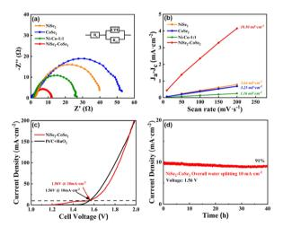
Fig. 6 (a) EIS measurements of prepared samples. (b)  $C_{\rm dl}$  values of prepared samples. (c) LSV measurements for overall water splitting performance of the devices based on NiSe2-CoSe2 electrodes and Pt/C + RuO<sub>2</sub> electrodes. (d) Chronoamperometric measurement of NiSe<sub>2</sub>-CoSe<sub>2</sub> aerogel toward overall water splitting
