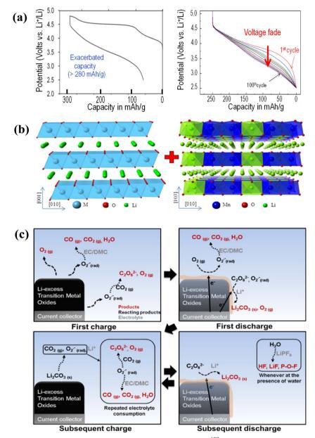
Fig. 7 (a) The first cycle charge-discharge curve of Li-rich manganese-based materials. 127 (b) Schematic diagram of the structure of Li<sub>2</sub>MnO<sub>3</sub>. 125 (c) Schematic diagram of the reaction mechanism of layered lithium excess metal oxides. 126
