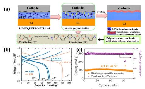
Fig. 11 (a) Electrochemical schematic diagram of the NCM<sub>523</sub>/PT-PEO-PT/Li battery.<sup>235</sup> (b) Formation of the conductive interface layer in a PEO battery.  $^{168}$  (c) Long cycle performance of the NCM<sub>523</sub>/PT-PEO-PT/Li battery at 40  $^{\circ}$ C.  $^{235}$
