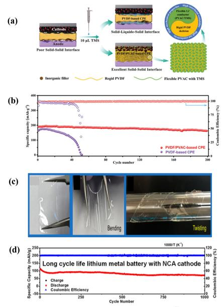
Fig. 9 (a) Schematic diagram of interface modification of a PVDF/PVAC solid electrolyte with TMS.<sup>179</sup> (b) Long cycle performance of a PVDF/PVAC battery.<sup>179</sup> (c) and (d) Photographs of the solid state electrolyte and long cycle performance diagram.<sup>180</sup>
