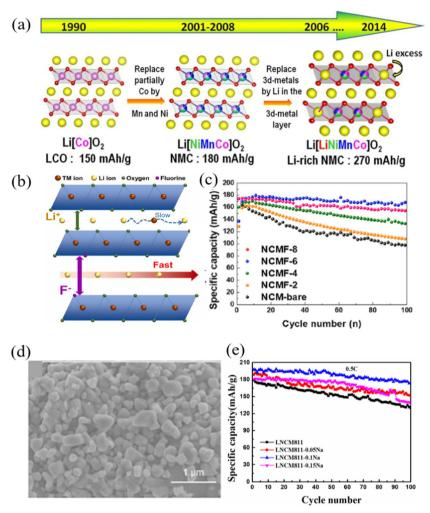
Fig. 5 (a) Schematic diagram of the structure of the ternary cathode material. 81 (b) and (c) Schematic diagram of the structural principle and cycle performance of F-modified NCM.<sup>84</sup> (d) and (e) Microscopy image and cycling performance of Na<sup>+</sup> doped and SiO<sub>2</sub> coated NCM.<sup>85</sup>
