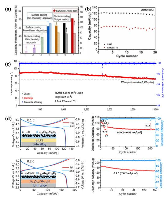
Fig. 8 (a) 5 V-class sulfurized spinel cathode stable in sulfide all-solid-state batteries. 172 (b) LNMOS<sub>0.15</sub> cycle performance diagram. 172 (c) Long cycle diagram of NCM<sub>85</sub> ASSLBs (performed after rate cycling) at a rate of 3C.<sup>173</sup> (d) Long cycle diagram of a lithium ytterbium halide solid electrolyte (LCO and NCM<sub>622</sub>).<sup>174</sup>
