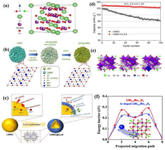
Fig. 6 (a) Schematic diagram of the structure of LNMO.<sup>118</sup> (b) Schematic diagram of LBO modification of LNMO.<sup>112</sup> (c) Schematic diagram of CuO modification of LNMO.<sup>114</sup> (d) The long cycle life of CuO-modified LNMO.<sup>114</sup> (e) Structures of ordered and disordered LiNi<sub>0.5</sub>Mn<sub>1.5</sub>O<sub>4</sub> with or without Cr doping. 115 (f) Schematic diagram of the structural principle of Cr-modified LNMO. 115
