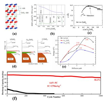
Fig. 4 (a) Schematic diagram of the structure of LiCoO<sub>2</sub>.<sup>63</sup> (b) Schematic diagram of LiCoO<sub>2</sub> delithiation phase transition.<sup>64</sup> (c) Change of the lattice constant c during LiCoO<sub>2</sub> delithiation.<sup>65</sup> (d) Energy levels of LiCoO<sub>2</sub> at different delithiation states.<sup>62</sup> (e) Decay of LiCoO<sub>2</sub>.<sup>63</sup> (f) Long cycle of MgF<sub>2</sub> modified LiCO2.66
