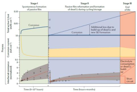
Fig. 13 Schematic diagram of corrosion of lithium in nonaqueous electrolytes, including ether-based or organic carbonate based electrolytes.<sup>259</sup>
