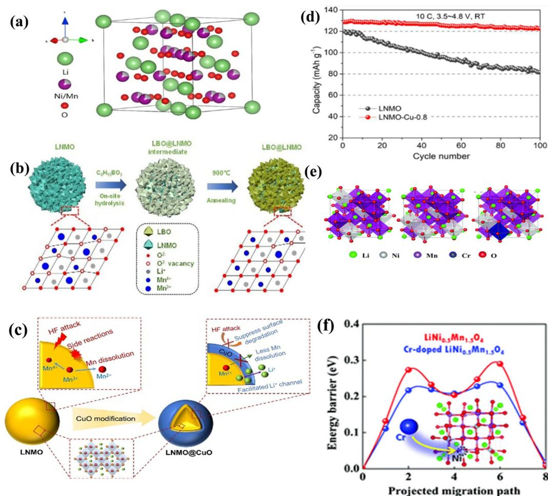
Fig. 6 (a) Schematic diagram of the structure of LNMO.<sup>118</sup> (b) Schematic diagram of LBO modification of LNMO.<sup>112</sup> (c) Schematic diagram of CuO modification of LNMO.<sup>114</sup> (d) The long cycle life of CuO-modified LNMO.<sup>114</sup> (e) Structures of ordered and disordered  $\text{LiNi}_{0.5}\text{Mn}_{1.5}\text{O}_4$  with or without Cr doping.<sup>115</sup> (f) Schematic diagram of the structural principle of Cr-modified LNMO.<sup>115</sup>
