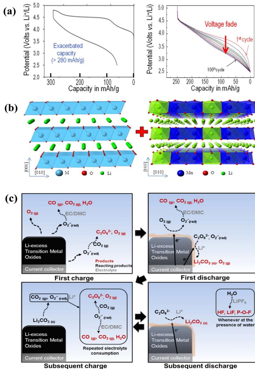
Fig. 7 (a) The first cycle charge–discharge curve of Li-rich manganese-based materials.<sup>127</sup> (b) Schematic diagram of the structure of  $\text{Li}_2\text{MnO}_3$ .<sup>125</sup> (c) Schematic diagram of the reaction mechanism of layered lithium excess metal oxides.<sup>126</sup>
