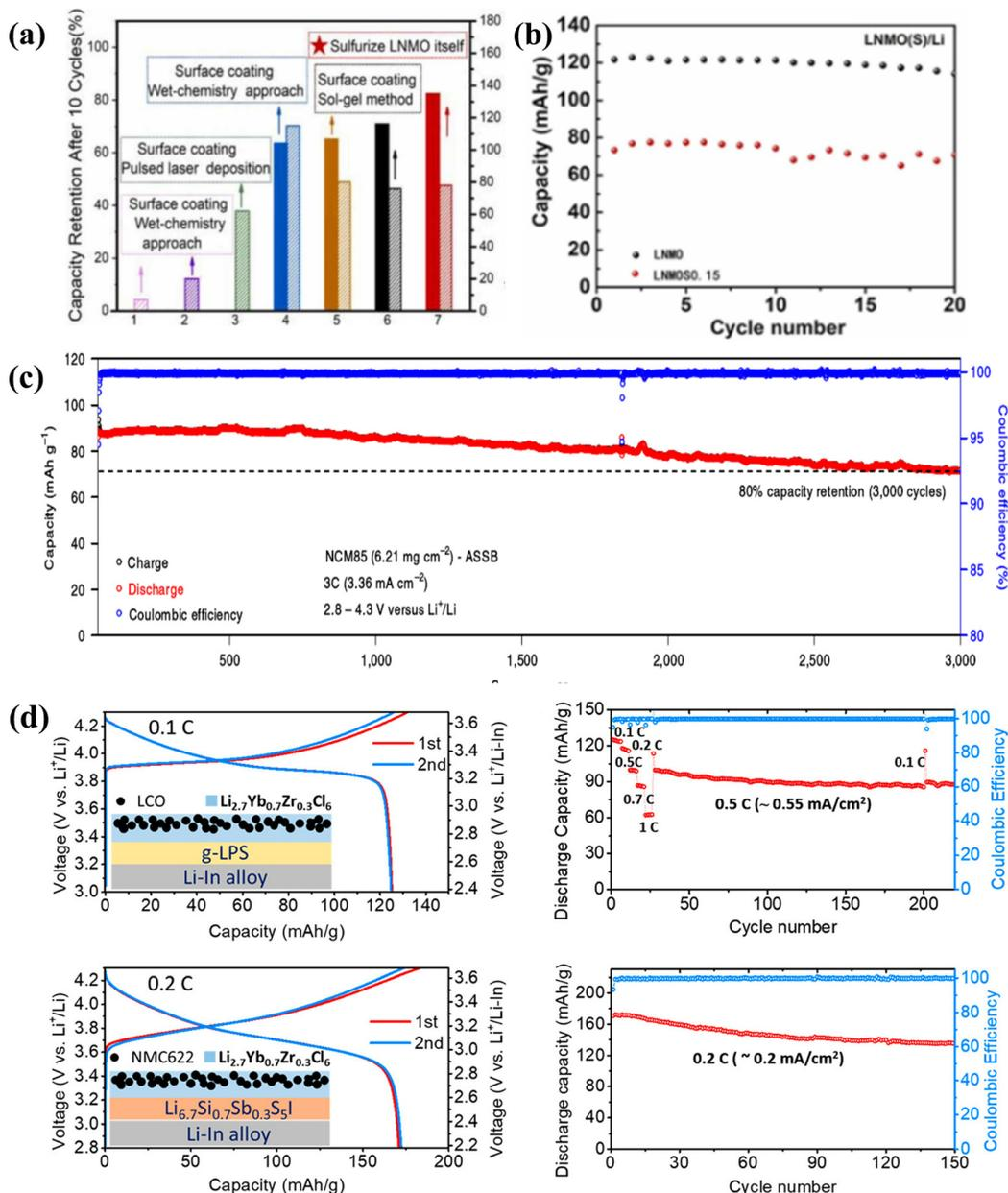
Fig. 8 (a) 5 V-class sulfurized spinel cathode stable in sulfide all-solid-state batteries.<sup>172</sup> (b) LNMO<sub>0.15</sub> cycle performance diagram.<sup>172</sup> (c) Long cycle diagram of NCM<sub>85</sub> ASSLBs (performed after rate cycling) at a rate of 3C.<sup>173</sup> (d) Long cycle diagram of a lithium ytterbium halide solid electrolyte (LCO and NCM<sub>622</sub>).<sup>174</sup>
