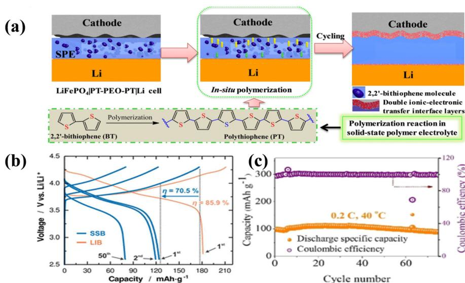
**Fig. 11** (a) Electrochemical schematic diagram of the  $\text{NCM}_{523}/\text{PT-PEO-PT}/\text{Li}$  battery.<sup>235</sup> (b) Formation of the conductive interface layer in a PEO battery.<sup>168</sup> (c) Long cycle performance of the  $\text{NCM}_{523}/\text{PT-PEO-PT}/\text{Li}$  battery at  $40^\circ\text{C}$ .<sup>235</sup>
