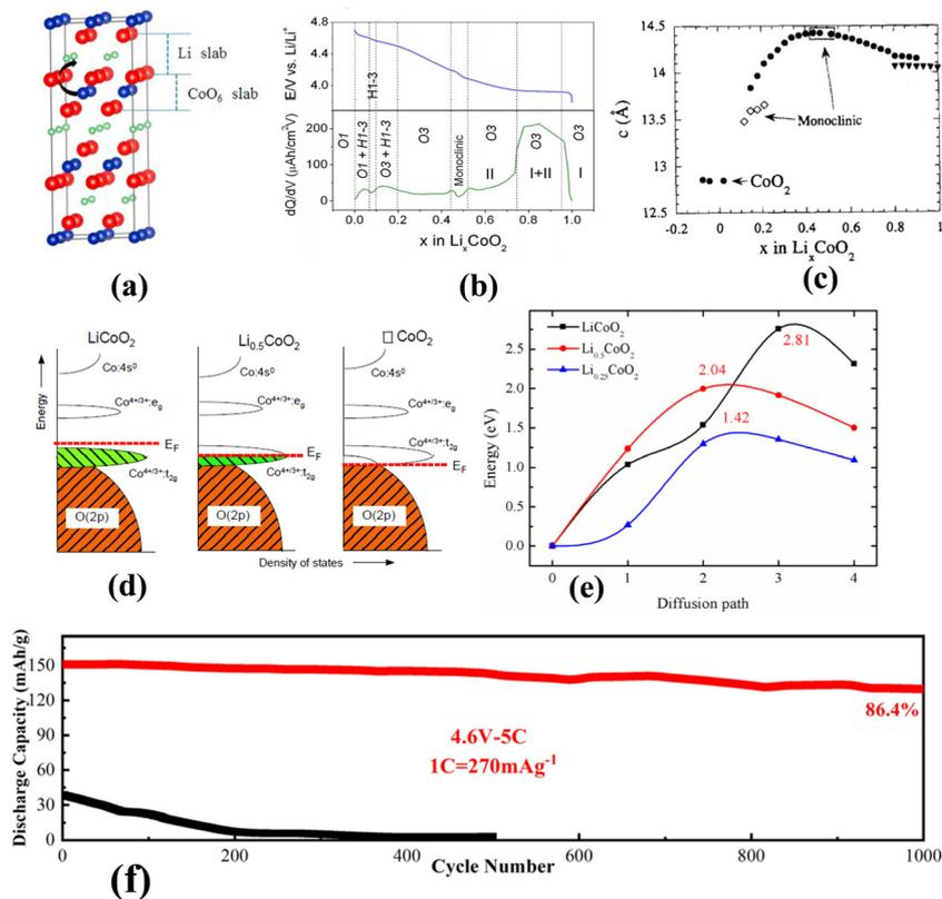
Fig. 4 (a) Schematic diagram of the structure of  $\text{LiCoO}_2$ .<sup>63</sup> (b) Schematic diagram of  $\text{LiCoO}_2$  delithiation phase transition.<sup>64</sup> (c) Change of the lattice constant  $c$  during  $\text{LiCoO}_2$  delithiation.<sup>65</sup> (d) Energy levels of  $\text{LiCoO}_2$  at different delithiation states.<sup>66</sup> (e) Decay of  $\text{LiCoO}_2$ .<sup>63</sup> (f) Long cycle of  $\text{MgF}_2$  modified  $\text{LiCoO}_2$ .<sup>66</sup>
