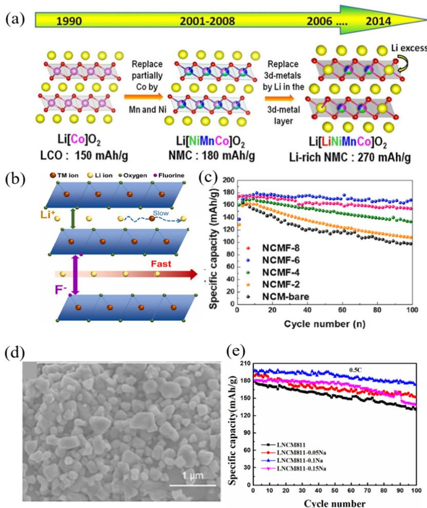
Fig. 5 (a) Schematic diagram of the structure of the ternary cathode material.<sup>81</sup> (b) and (c) Schematic diagram of the structural principle and cycle performance of F-modified NCM.<sup>84</sup> (d) and (e) Microscopy image and cycling performance of Na<sup>+</sup> doped and SiO<sub>2</sub> coated NCM.<sup>85</sup>
