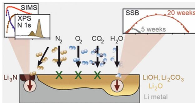
Fig. 14 Diagram of the reaction interface between Li and different substances.<sup>260</sup>
