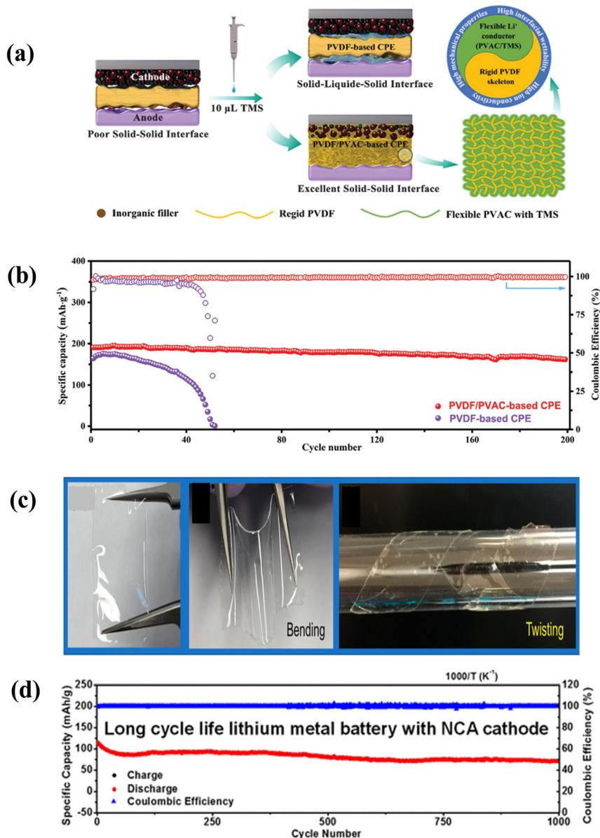
Fig. 9 (a) Schematic diagram of interface modification of a PVDF/PVAC solid electrolyte with TMS.<sup>179</sup> (b) Long cycle performance of a PVDF/PVAC battery.<sup>179</sup> (c) and (d) Photographs of the solid state electrolyte and long cycle performance diagram.<sup>180</sup>
