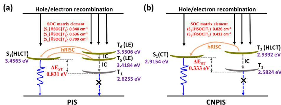
Fig. 3 Probable emission mechanism based on the HLCT state for **PIS** (a) and **CNPIS** (b). S and T are singlet and triplet excited states; LE and CT represent local excited and charge-transfer states;  $\Delta E_{\text{ST}}$  is the singlet-triplet energy splitting between  $S_1$  and  $T_1$ ; IC and hRISC are the internal conversion and the high-lying reverse intersystem crossing.
