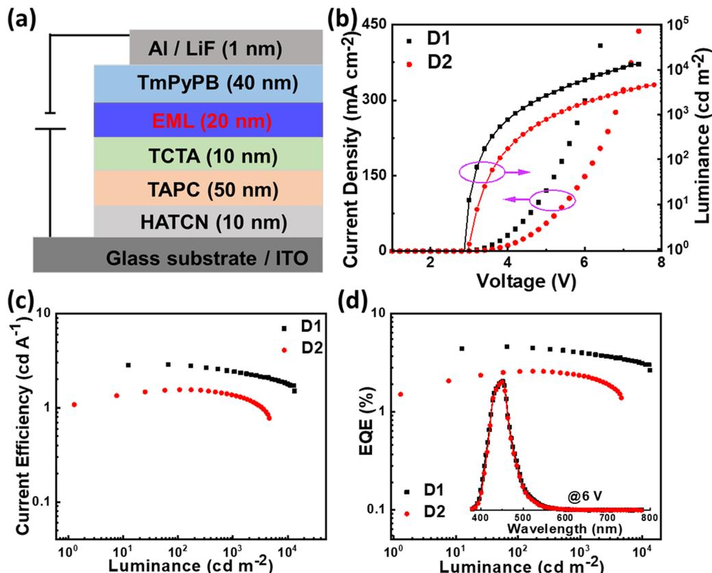
Fig. 4 (a) Device configuration diagram. (b) Current–density–voltage–luminance characteristics of the fabricated OLEDs (**D1** and **D2**). (c) Current efficiency versus luminance curves of devices **D1** and **D2**. (d) EQE versus luminance curves of devices **D1** and **D2**. Inset: Normalized EL spectra at the voltage of 6 V.
