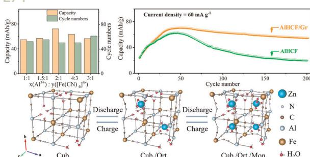
Open-framework aluminum hexacyanoferrate as a cathode material for high voltage aqueous zinc-ion batteries: effect of Al<sup>3+</sup> cations on three-phase transition of AlFe(CN)<sub>6</sub>
