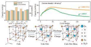
Open-framework aluminum hexacyanoferrate as a cathode material for high voltage aqueous zinc-ion batteries: effect of Al<sup>3+</sup> cations on three-phase transition of AlFe(CN)6
