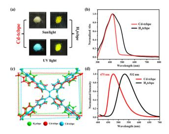
Fig. 2 (a) Emissive photographs of Cd-tcbpe and H4tcbpe under a hand UV light of 365 nm; (b) UV-vis spectra of Cd-tcbpe-B and H<sub>4</sub>tcbpe ligand; (c) comparison of tcbpe linkers in Cd-tcbpe (red, blue) and  $H_4$ tcbpe (green); (d) fluorescence emission spectra of **Cd-tcbpe** ( $\lambda_{ex}$  = 370 nm) and H<sub>4</sub>tcbpe ( $\lambda_{ex}$  = 390 nm).
