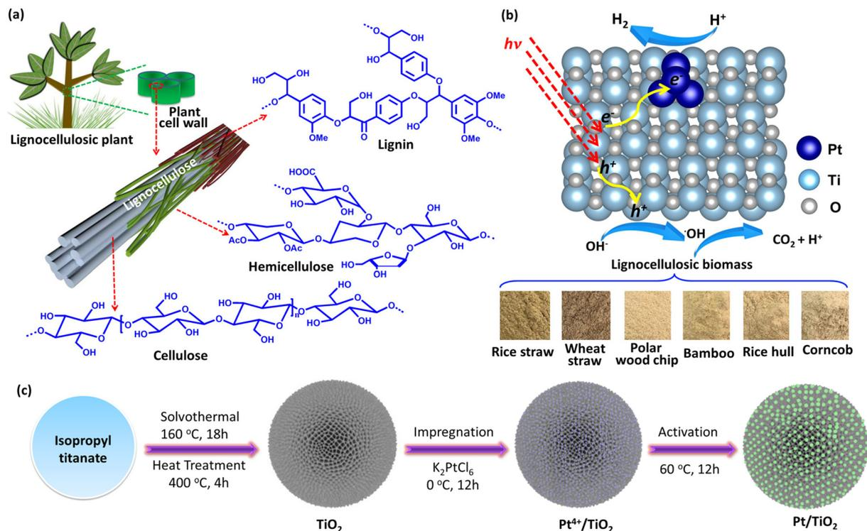
**Fig. 1** (a) Chemical composition and structure of lignocellulosic biomass. (b) Photocatalytic H<sub>2</sub> production from lignocellulosic biomass over Pt nanocluster anchored porous TiO<sub>2</sub> microspheres photocatalysts. (c) Schematic illustration for the synthesis of Pt/TiO<sub>2</sub> photocatalysts.
