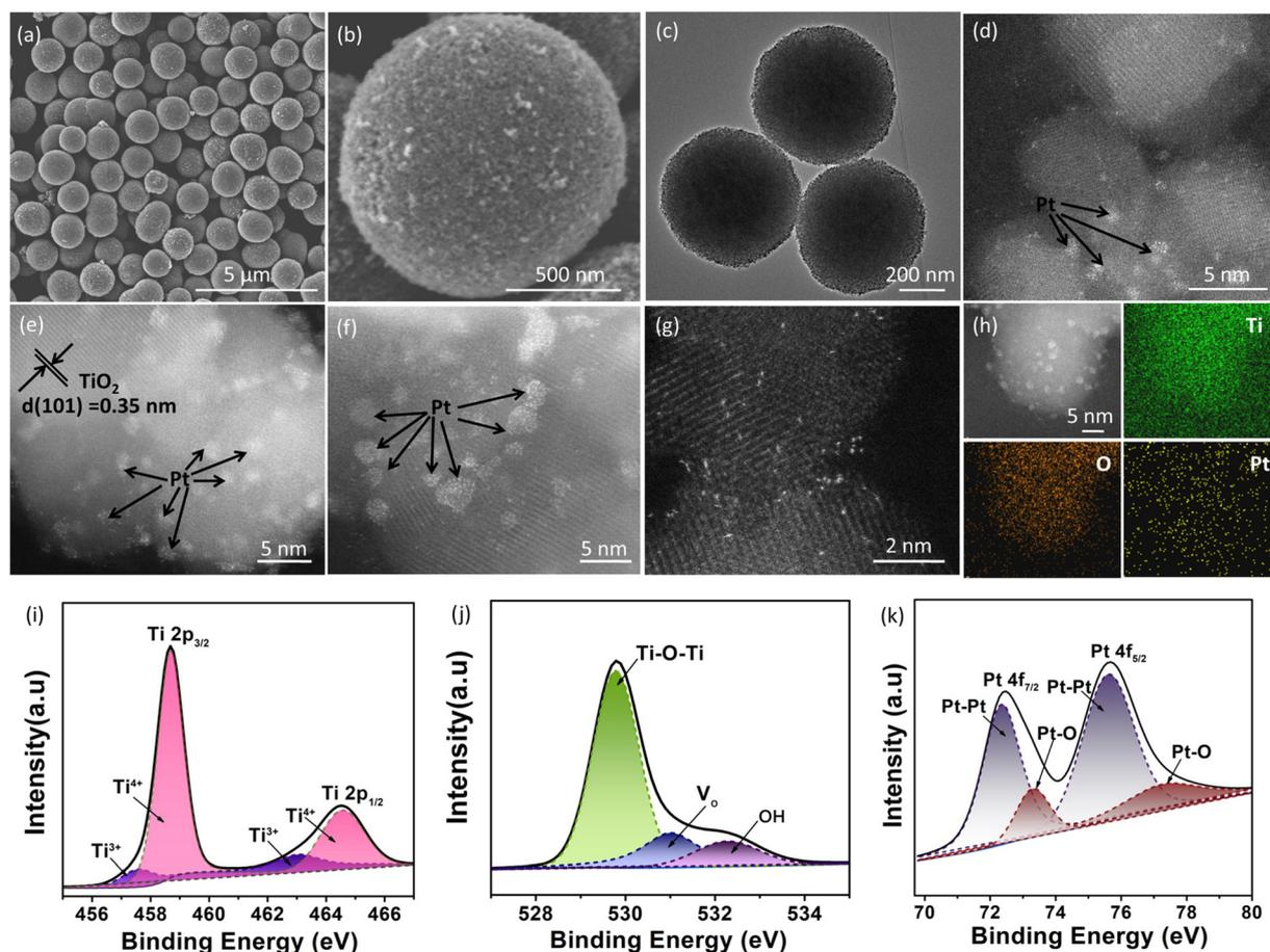
**Fig. 2** (a and b) SEM and (c) TEM image of bare  $\text{TiO}_2$ . (d–g) Spherical aberration-corrected HAADF-STEM image of 0.2%  $\text{Pt}/\text{TiO}_2$  (d), 0.4%  $\text{Pt}/\text{TiO}_2$  (e and g) and 1.0%  $\text{Pt}/\text{TiO}_2$  (f). (h) HAADF-STEM and elemental mapping images of 0.4%  $\text{Pt}/\text{TiO}_2$ . (i–k) High-resolution Ti 2p, O 1s and Pt 4f XPS spectra of 0.4%  $\text{Pt}/\text{TiO}_2$ .
