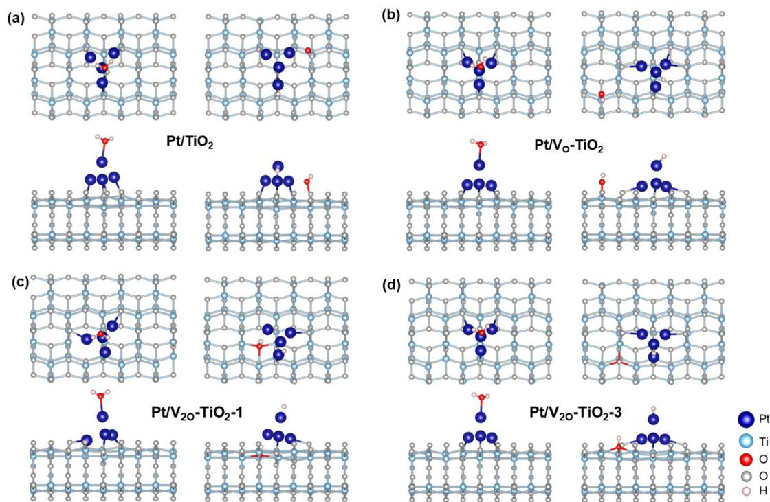
Fig. 6 Structures for  $^*H_2O$  and  $^*OH/^*H$  adsorbed on the (a) Pt/TiO<sub>2</sub>, (b) Pt/V<sub>O</sub>-TiO<sub>2</sub>, (c) Pt/V<sub>20</sub>-TiO<sub>2</sub>-1, (d) Pt/V<sub>20</sub>-TiO<sub>2</sub>-3 surfaces.
