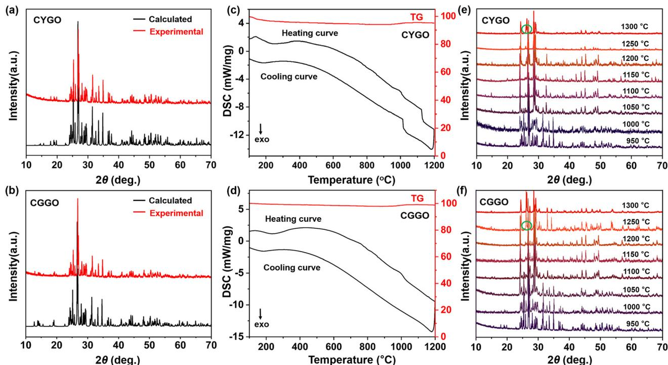
**Fig. 1** (a and b) Experimental and theoretical PXRD patterns of CYGO and CGGO; (c and d) TG-DSC curves of CYGO and CGGO; (e and f) the PXRD patterns evolution of CYGO and CGGO polycrystalline pure phases under elevated temperature conditions.
