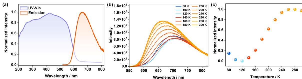
**Fig. 2** (a) UV-vis absorption and emission spectra (excited at 365 nm) of CIPP in air at room temperature. (b) Temperature-dependent emission spectra of CIPP, from 80 K to 300 K, excited at 365 nm. (c) A scatter plot of the integral emission intensity of CIPP at the corresponding temperature, based on (b).
