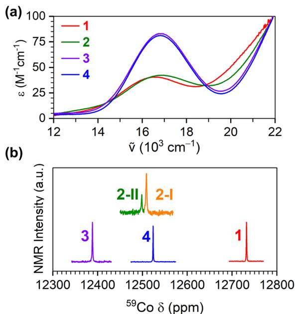
**Fig. 3** Characterization of Co(III) electronic structure in 1–4. (a) UV-vis spectra for 1–4 in  $\text{CH}_2\text{Cl}_2$  at room temperature, focused on the d-d transition. (b)  $^{59}\text{Co}$  NMR spectra (ca. 118.3 MHz) for 1–4 in  $\text{CDCl}_3$  at room temperature. Spectra were collected in a 500 MHz  $^1\text{H}$  magnet (11.7 T).
