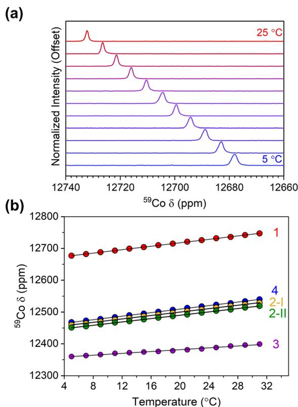
**Fig. 4** (a) Variable-temperature  $^{59}\text{Co}$  NMR for **1** in  $\text{CDCl}_3$  at 100 mM concentration. (b) Peak positions for **1–4** as a function of temperature at 100 mM concentration in  $\text{CDCl}_3$ .
