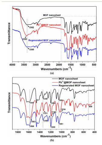
**Fig. 8** Comparison of the FT-IR spectra at  $400-4000~\text{cm}^{-1}$  (a) and  $400-1900~\text{cm}^{-1}$  (b) for MOF nanosheets, Pb<sup>2+</sup>@MOF nanosheets, and regenerated MOF nanosheets.
