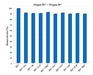
Fig. 7 Effect of the coexistent ions (50 ppm) on Pb<sup>2+</sup> (10 ppm) removal by MOF nanosheets.
