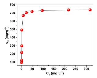
Pb<sup>2+</sup> adsorption isotherm for MOF nanosheets.
