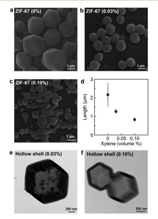
Fig. 4 (a-c) SEM images of ZIF-67 crystals generated by the addition of microemulsion with different volume ratios of xylene (a: 0%, b: 0.03% and c: 0.10%). (d) ZIF-67 crystal size as a function of xylene volume (left: 0%, middle: 0.03% and right: 0.10%). TEM images of hollow nanostructures made from ZIF-67 crystals produced using (e) the 0.03% xylene-based microemulsion and (f) the 0.10% xylene-based microemulsion.
