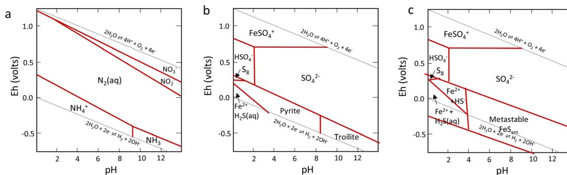
**Fig. 3** Key Pourbaix diagrams of relevance to this work. (a) Shows the nitrogen system, (b) the Fe/S system with thermodynamically stable products, and (c) the Fe/S system with metastable mackinawite shown. Reproduced from ref. 96 with permission from John Wiley and Sons, copyright 2022.
