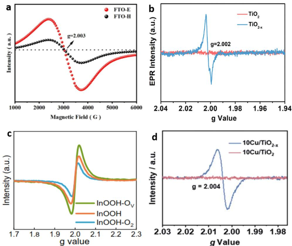
**Fig. 5** Displays the EPR spectra of (a) FTO prepared by electrospinning and hydrothermal methods. Reproduced from ref. 103 with permission from Wiley, copyright 2022. (b) Pristine  $\text{TiO}_2$  and  $\text{TiO}_{2-x}$  nanotubes. Reproduced from ref. 105 with permission from the American Chemical Society, copyright 2020. (c) Indium oxyhydroxide with different vacancies. Reproduced from ref. 22, and (d) Cu cluster deposited  $\text{TiO}_2$ . Reproduced from ref. 106.
