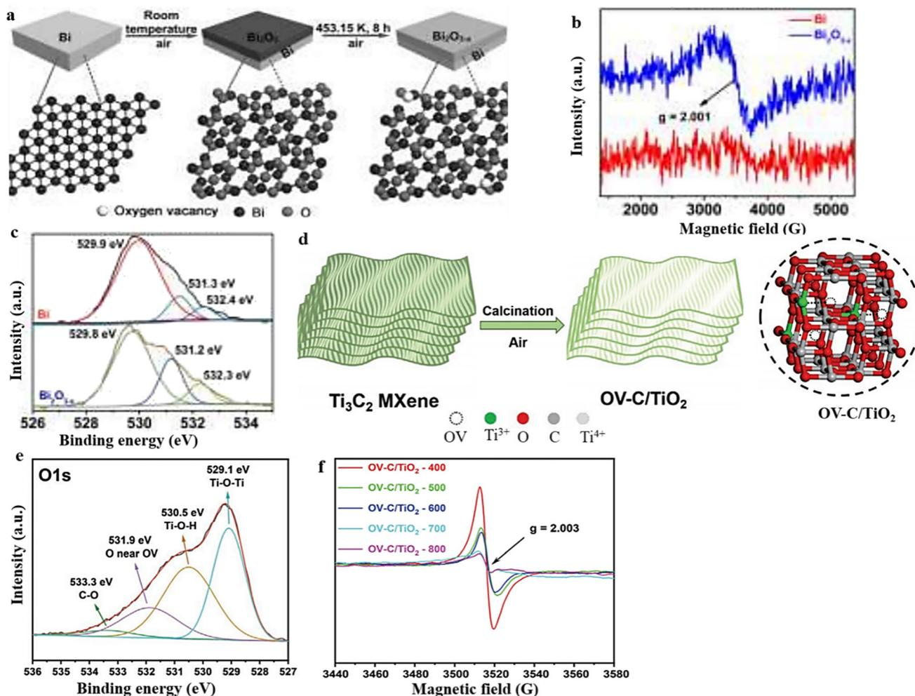
**Fig. 8** (a) An illustration of the schematic process for the production of a layer of  $\text{Bi}_2\text{O}_{3-x}$  with oxygen vacancies. (b) and (c) EPR and O 1s XPS spectra of  $\text{Bi}_2\text{O}_{3-x}$ . Reproduced from ref. 127 with permission from Wiley, copyright 2020. (d) Diagram of the preparation process of OV-C/ $\text{TiO}_2$ . (e) and (f) The O 1s XPS and EPR spectra of OV-C/ $\text{TiO}_2$ . Reproduced from ref. 130 with permission from Wiley, copyright 2021.
