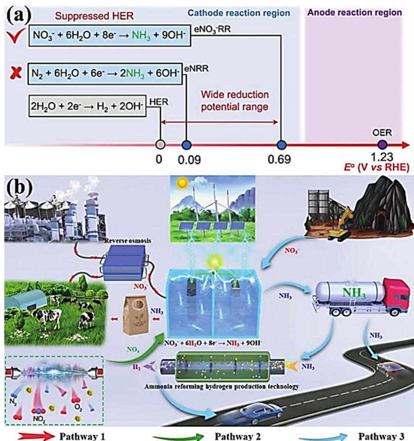
**Fig. 1** (a) The standard reduction potentials for the HER, NRR, and NO<sub>3</sub>RR were compared. Reproduced from ref. 29 with permission from the American Chemical Society, copyright 2022. (b) The design schematic illustration of the NO<sub>3</sub>RR process to NH<sub>3</sub>. Reproduced from ref. 33 with permission from Wiley, copyright 2023.
