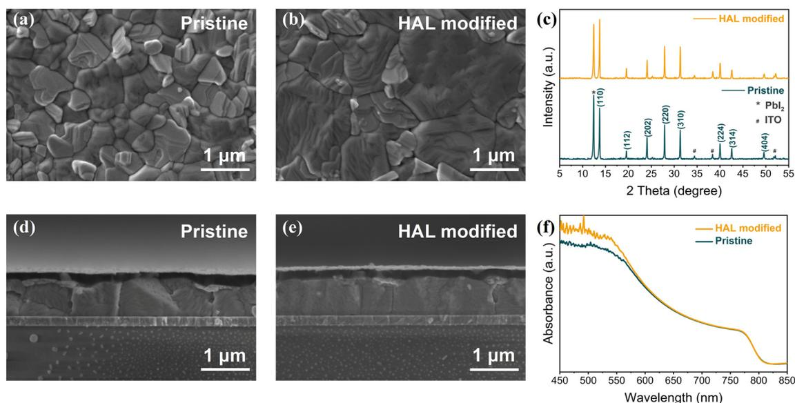
**Fig. 2** Top-view SEM images of PVK films with (a) pristine and (b) HAL-modified SnO<sub>2</sub> films. (c) XRD patterns and (f) UV-Vis absorption spectra of PVK films with different SnO<sub>2</sub> films. Cross-sectional SEM images of PSC devices with (d) pristine and (e) HAL-modified SnO<sub>2</sub> films.
