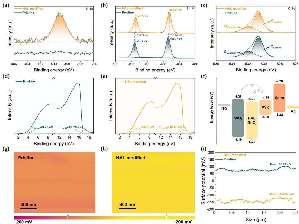
**Fig. 1** (a) N 1s, (b) Sn 3d, and (c) O 1s XPS spectra of different SnO<sub>2</sub> films. UPS spectra of (d) SnO<sub>2</sub> and (e) HAL-modified SnO<sub>2</sub> films. (f) Energy band diagram of the materials employed in PSCs. KPFM images of (g) SnO<sub>2</sub> and (h) HAL-modified SnO<sub>2</sub> films. (i) Surface potential of different SnO<sub>2</sub> films.
