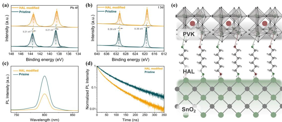
**Fig. 3** (a) Pb 4f and (b) I 3d XPS spectra of  $\text{PbI}_2$  films based on different  $\text{SnO}_2$  films. (c) SSPL and (d) TRPL spectra of PVK films based on different  $\text{SnO}_2$ . (e) Schematic diagram illustrating potential interaction mechanisms for the buried interfacial modification of HAL.
