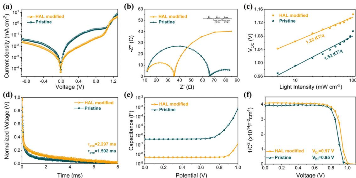
**Fig. 4** (a) The dark-state  $J$ - $V$  curves, (b) Nyquist plots, (c) Light-intensity-dependent  $V_{OC}$  curves, (d) TPV curves, (e)  $C$ - $V$  curves, and (f)  $M$ - $S$  curves for PSCs based different  $\text{SnO}_2$  films.
