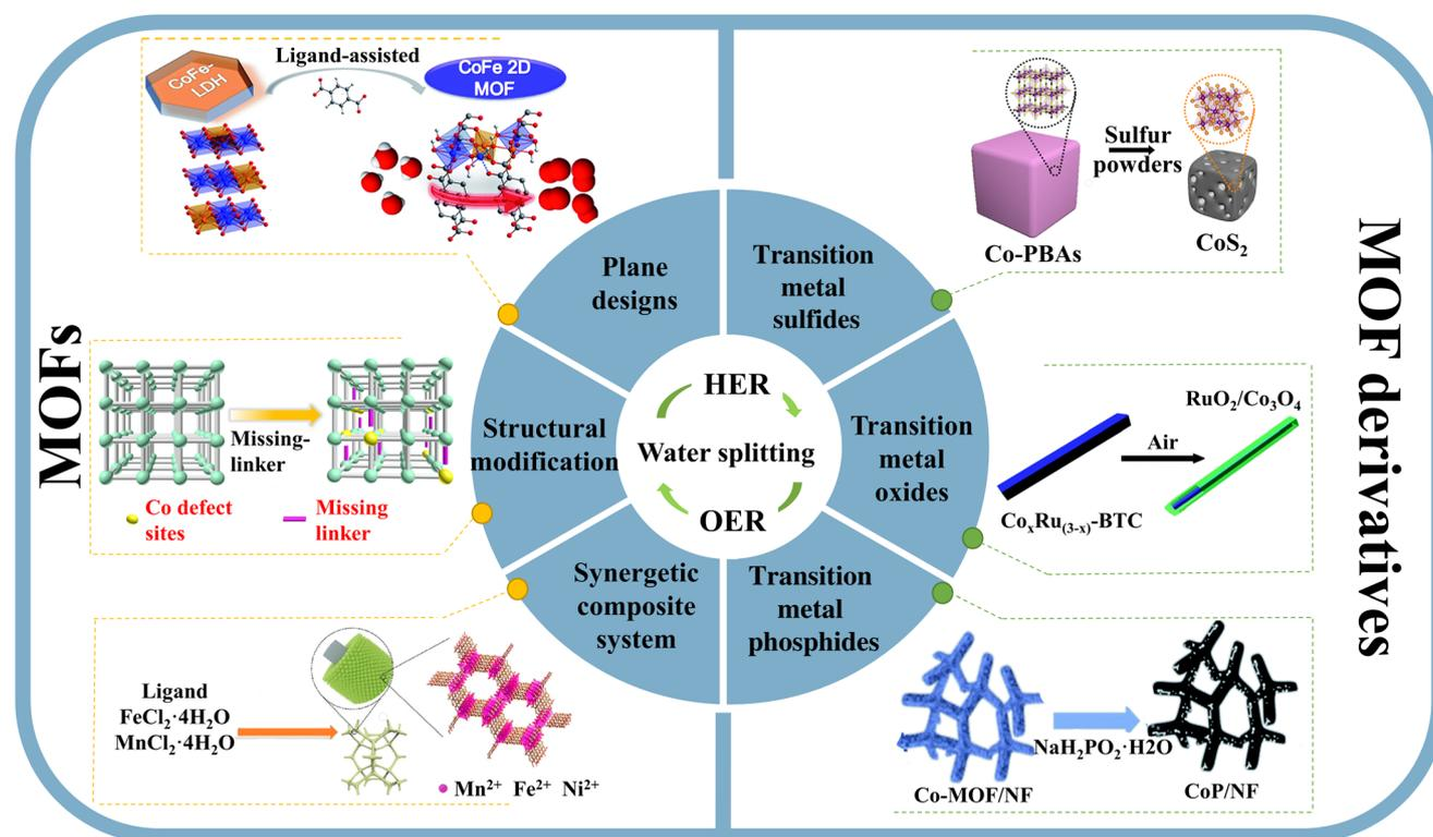
**Scheme 1** Illustration of the main design strategies and types of MOFs and MOF derivatives in water splitting. Reproduced with permission.<sup>60,66,75,83,88,91</sup> Copyright 2019, RSC. Copyright 2019, Springer Nature. Copyright 2020, Wiley-VCH. Copyright 2017, RSC. Copyright 2017, RSC. Copyright 2020, RSC.
