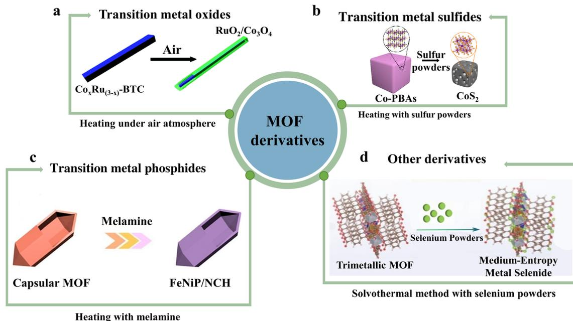
**Fig. 4** Illustration of MOF derivatives including (a) transition metal oxides, (b) transition metal sulfides, (c) transition metal phosphides and (d) other derivatives in electrocatalytic water splitting. Reproduced with permission.<sup>83,88,94,100</sup> Copyright 2017, RSC. Copyright 2019 Springer Nature. Copyright 2020, RSC. Copyright 2019, American Chemical Society.
