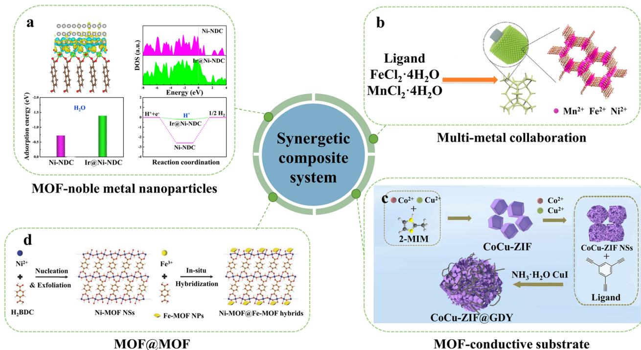
**Fig. 3** Illustration of the synergetic composite system of MOF-based materials in electrocatalytic water splitting, (a) MOF-noble metal nanoparticles, (b) multi-metal collaboration, (c) MOF-conductive substrate and (d) MOF@MOF. Reproduced with permission<sup>70,71,75,76</sup> Copyright 2023, Wiley-VCH. Copyright 2020, Wiley-VCH. Copyright 2020 Elsevier. Copyright 2018, Wiley-VCH.
