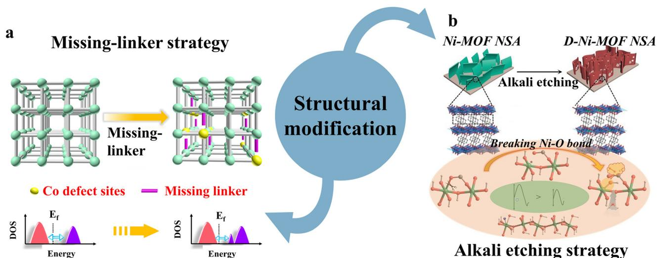
**Fig. 2** Illustration of the structural modification strategies of MOF-based materials in electrocatalytic water splitting. (a) missing-linker strategy and (b) alkali etching strategy. Reproduced with permission.<sup>66,67</sup> Copyright 2020, Wiley-VCH. Copyright 2019 Springer Nature.
