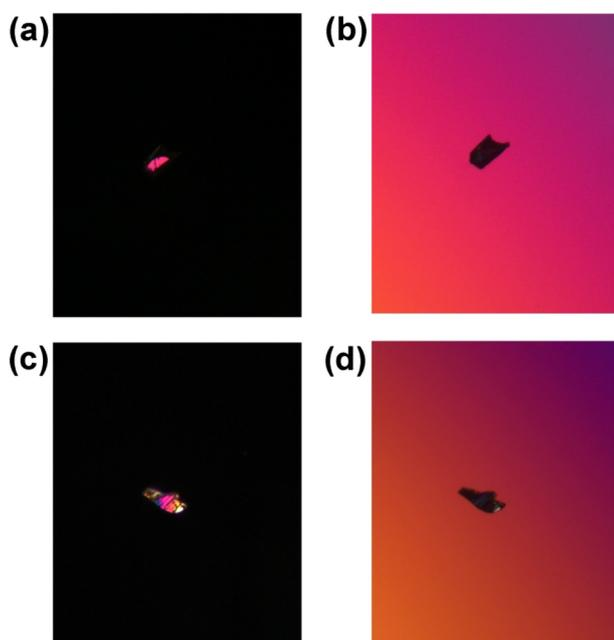
**Fig. 3** (a and b)  $\text{Ba}_3\text{MnGe}_3\text{O}_2\text{S}_8$  and (c and d)  $\text{Ba}_3\text{CdGe}_3\text{O}_2\text{S}_8$  crystals for birefringence determination and the interference colors observed before and after complete extinction.
