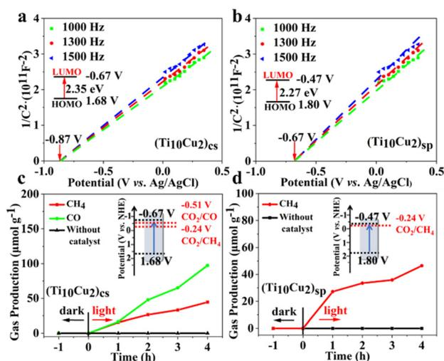
Fig. 5 Mott–Schottky plots of  $(\text{Ti}_{10}\text{Cu}_2)_{\text{cs}}$  (a) and  $(\text{Ti}_{10}\text{Cu}_2)_{\text{sp}}$  (b). Time courses of photocatalytic  $\text{CO}_2$  reduction using  $(\text{Ti}_{10}\text{Cu}_2)_{\text{cs}}$  (c),  $(\text{Ti}_{10}\text{Cu}_2)_{\text{sp}}$  (d) and their band structure diagrams.
