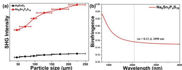
**Fig. 5** (a) Powder SHG response versus particle size in  $\text{Na}_6\text{Sn}_3\text{P}_4\text{S}_{16}$  with  $\text{AgGaS}_2$  as a reference. (b) Calculated birefringence in  $\text{Na}_6\text{Sn}_3\text{P}_4\text{S}_{16}$ .
