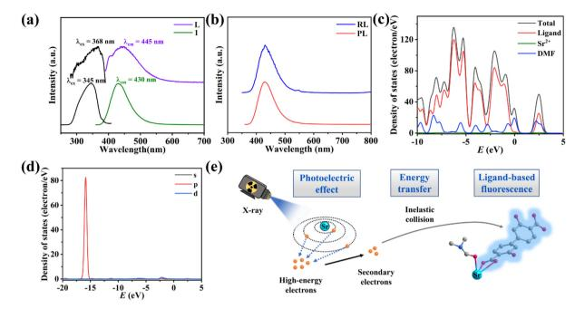
Fig. 4 (a) The solid-state PL excitation and emission spectra of H<sub>2</sub>DOBPDC and 1. (b) The PL and RL spectra of 1. (c) Profile of the total/partial electronic density of states of 1. (d) The partial electronic density of states of  $Sr^{2+}$ . (e) Diagram of the RL mechanism of 1.
