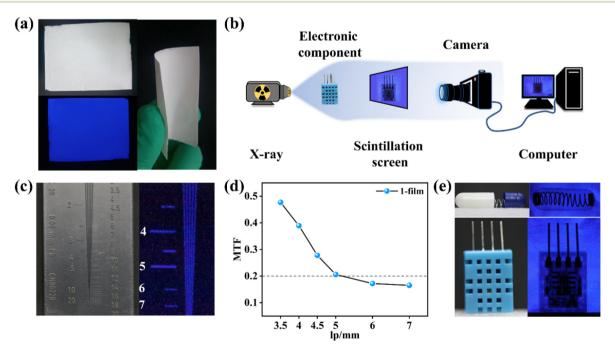
Fig. 5 (a) The photographs of the flexible 1-film. (b) The schematic diagram of the self-built X-ray imaging system. (c) Photograph of real line pair card and its X-ray radiograph. (d) The MTF value of the 1-film by the line-pair pattern method. (e) The real pictures and X-ray radiographs of the capsule and electronic component.
