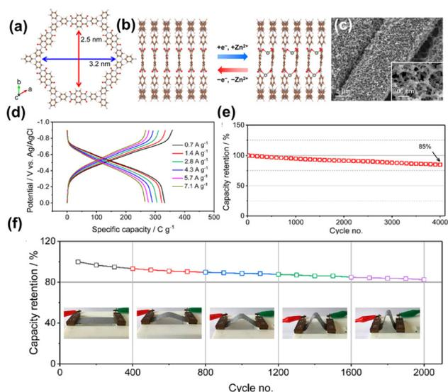
**Fig. 16** (a) 2D PI-COF structure. (b) Zn<sup>2+</sup>-storage process in PI COF. (c) SEM images for PI-COF. (d) Charge/discharge curves. (e) Cycling performance of the PI-COF electrode at  $10 \text{ mV s}^{-1}$ . (f) Cycling performance of PI-COF//MnO<sub>2</sub> battery at  $0.1 \text{ V s}^{-1}$  in different deformation states. Reproduced from ref. 48 with permission from American Chemical Society, copyright 2020.
