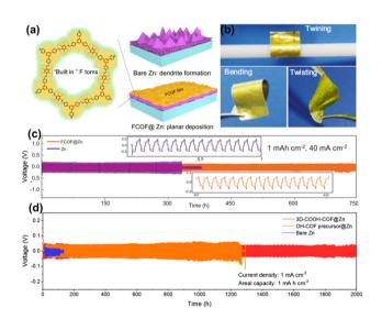
Fig. 11 (a) Mechanism comparison of the Zn deposition processes. (b) Pictures of flexibility FCOF. (c) Stability test for Zn symmetric cells at 1 mA h cm<sup>-2</sup>, 40 mA cm<sup>-2</sup>. Reproduced from ref. 38 with permission from Springer Nature, copyright 2021. (d) Long-term cycling performance of Zn plating/stripping in symmetric cells. Reproduced from ref. 39 with permission from Elsevier Inc., copyright 2022.
