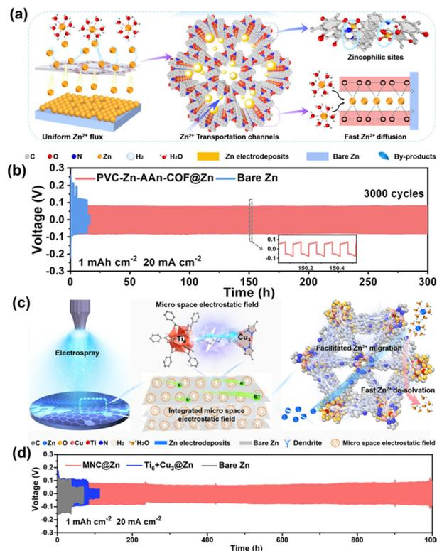
**Fig. 12** (a) Mechanism comparison of the Zn deposition on Zn-COF@Zn anode. (b) Cycling stability of symmetrical cells on bared Zn and PVC-Zn-AAn-COF@Zn. Reproduced from ref. 55 with permission from John Wiley & Sons, copyright 2022. (c) Schematic of electro spray preparation process of MNC for ZMBs Zn coating. (d) Cycling stability of a symmetric cell. Reproduced from ref. 86 with permission from John Wiley & Sons, copyright 2023.
