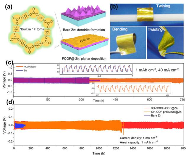
**Fig. 11** (a) Mechanism comparison of the Zn deposition processes. (b) Pictures of flexibility FCOF. (c) Stability test for Zn symmetric cells at  $1 \text{ mA h cm}^{-2}$ ,  $40 \text{ mA cm}^{-2}$ . Reproduced from ref. 38 with permission from Springer Nature, copyright 2021. (d) Long-term cycling performance of Zn plating/stripping in symmetric cells. Reproduced from ref. 39 with permission from Elsevier Inc., copyright 2022.
