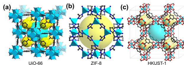
**Fig. 2** Crystal structures of (a) UiO-66, reproduced from ref. 28 with permission from American Chemical Society, copyright 2008. (b) ZIF-8, reproduced from ref. 29 with permission from Proceedings of the National Academy of Sciences of the United States of America, copyright 2006. (c) HKUST-1, reproduced from ref. 30 with permission from American Association for the Advancement of Science, copyright 1999.
