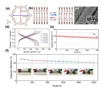
Fig. 16 (a) 2D PI-COF structure. (b) Zn<sup>2+</sup>-storage process in PI COF. (c) SEM images for PI-COF. (d) Charge/discharge curves. (e) Cycling performance of the PI-COF electrode at 10 mV s<sup>-1</sup>. (f) Cycling performance of PI-COF//MnO<sub>2</sub> battery at 0.1 V s<sup>-1</sup> in different deformation states. Reproduced from ref. 48 with permission from American Chemical Society, copyright 2020.
