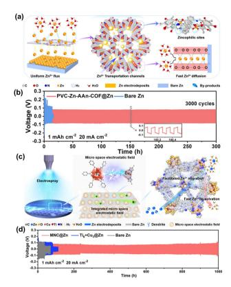
Fig. 12 (a) Mechanism comparison of the Zn deposition on Zn-COF@Zn anode. (b) Cycling stability of symmetrical cells on bared Zn and PVC-Zn-AAn-COF@Zn. Reproduced from ref. 55 with permission from John Wiley & Sons, copyright 2022. (c) Schematic of electrospray preparation process of MNC for ZMBs Zn coating. (d) Cycling stability of a symmetric cell. Reproduced from ref. 86 with permission from John Wiley & Sons, copyright 2023.
