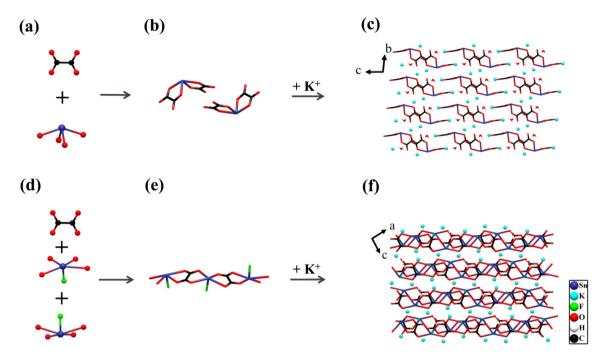
Fig. 1 (a and d) The coordination modes of  $Sn^{2+}$  and planar  $[C_2O_4]^{2-}$  groups; (b and e) the different connection modes between  $Sn^{2+}$ -polyhedra and  $[C_2O_4]^{2-}$  groups; (c and f) the structure of  $K_2Sn(C_2O_4)_2 \cdot H_2O$  and  $K_2Sn_2(C_2O_4)_2 \cdot H_2O$  along the a-axis and b-axis, respectively.
