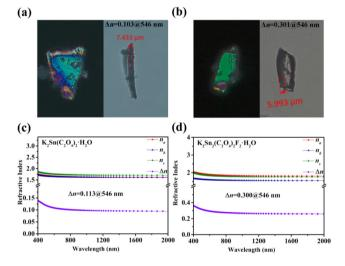
Fig. 2 (a and b) Experimental birefringence at 546 nm; (c and d) calculated refractive index for  $K_2Sn(C_2O_4)_2 \cdot H_2O$  and  $K_2Sn_2(C_2O_4)_2F_2 \cdot H_2O$ .
