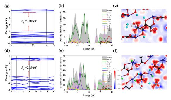
Fig. 5 (a and d) Calculated band structures; (b and e) total and partial density of states; and (c and f) electron density difference maps for K<sub>2</sub>Sn  $(C_2O_4)_2 \cdot H_2O$  and  $K_2Sn_2(C_2O_4)_2F_2 \cdot H_2O$ .
