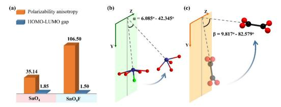
Fig. 4 (a) The polarizability anisotropy and HOMO-LUMO gap of  $Sn^{2+}$ -polyhedra ( $SnO_4$  for  $K_2Sn(C_2O_4)_2 \cdot H_2O$  and  $SnO_4F$  for  $K_2Sn_2(C_2O_4)_2 \cdot H_2O$ ); (b) the angles between the lone pair electron of  $Sn^{2+}$  and the YZ plane; and (c) the dihedral angles between the  $[C_2O_4]^{2-}$  plane and YZ plane in  $K_2Sn$  $(C_2O_4)_2 \cdot H_2O$  and  $K_2Sn_2(C_2O_4)_2F_2 \cdot H_2O$ .
