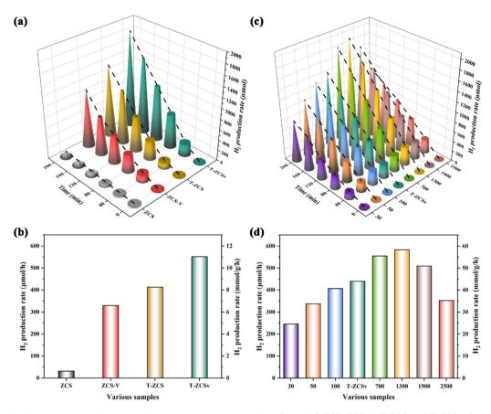
Fig. 9 Photocatalytic hydrogen production performance for various samples: (a and b) ZCS, ZCS-V, T-ZCS and T-ZCSv; (c and d) a series of ZIF-8@T-ZCSv composites with different contents.
