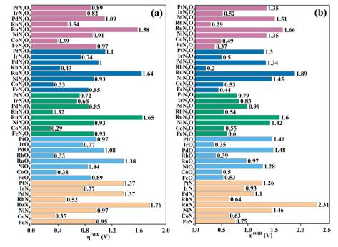
Fig. 3 Calculated (a) OER and (b) ORR overpotentials of different designed TMN<sub>x</sub>O<sub>4-x</sub>-HTC catalysts.
