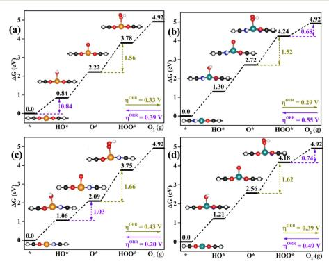
Fig. 4 Calculated free energy diagrams of the promising bifunctional catalysts for the OER and ORR: (a)  $RhO_4$ -HTC, (b)  $CoN_3O_1$ -HTC, (c)  $RhN_2O_2$ -HTC and (d) CoN<sub>1</sub>O<sub>3</sub>-HTC. The yellow and pink values are the potential-determining step values for the OER and ORR. The optimized configurations of intermediates on the catalysts are also exhibited.
