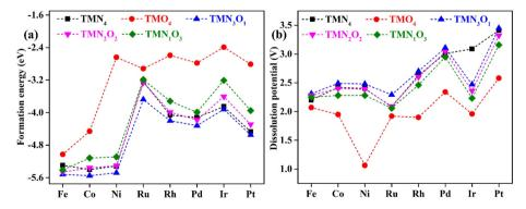
Fig. 2 Calculated (a) formation energy and (b) dissolution potential of transition metal atoms for the designed TMN<sub>x</sub>O<sub>4-x</sub>-HTC catalysts.
