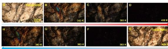
**Fig. 5** Evolutions of the ferroelastic domains under the polarizing microscope. (A) Natural optical microscope image for a single crystal of **1** in LTP, (B–D) evolutions of the ferroelastic domain structure for **1** in the heating, (E) natural optical microscope image for single crystal **1** in HTP, (F–H) and ferroelastic domain evolutions of **1** in the cooling process.
