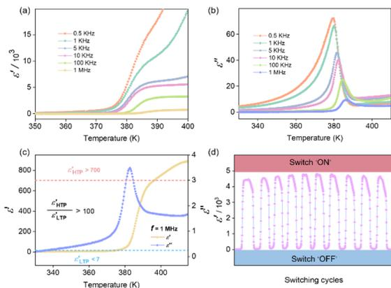
**Fig. 4** The dielectric anomaly measurement of polycrystalline samples of **1**. (a)  $\epsilon'$  at different frequencies upon heating. (b)  $\epsilon''$  at different frequencies upon heating. (c)  $\epsilon'$  and  $\epsilon''$  at 1 MHz. (d) After 10 switching cycles at a frequency of 25 kHz, the value of the dielectric constant shows a sensitive switchable with no decrease.
