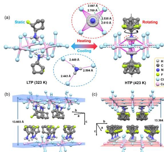
**Fig. 2** (a) Dipole rotor TFCA reorientation and interaction changes of **1** between 323 K (LTP) and 423 K (HTP). (b) and (c) The molecular structural packing model in LTP and HTP of **1** (some of the hydrogen atoms have been omitted for clarity).
