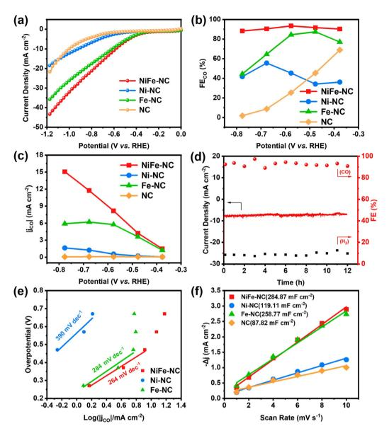
Fig. 3 (a) LSV curves of the prepared catalysts measured in CO<sub>2</sub>-saturated 0.5 M KHCO<sub>3</sub> electrolyte; (b) FE<sub>CO</sub> and (c) CO partial current density of the prepared catalysts; (d) stability test for NiFe-NC at -0.58 V vs. RHE with 12 h of continuous electrolysis; (e) Tafel plots for the CO partial current density of different samples; and (f) the electrochemical double-layer capacitances of different samples.
