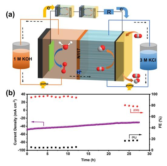
Fig. 6 (a) Schematic diagram of a self-driven CO<sub>2</sub> flow electrolysis system powered by two-series-connected homemade ZABs and (b) the current density and FE results in the self-driven CO<sub>2</sub> flow electrolysis systems.
