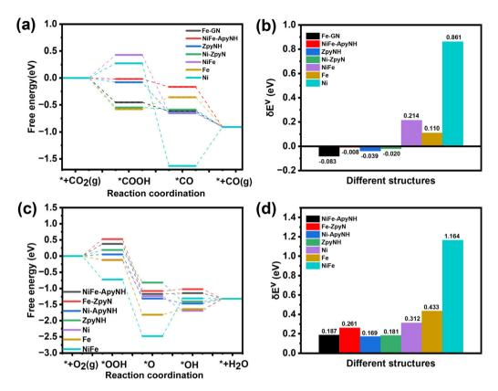
Fig. 7 The free energy diagrams (FEDs) of  $CO_2RR$  (a) and ORR (c) on optimal active site for each type; (b) the  $\delta E^{\nu}$  values of  $CO_2RR$  (b) and ORR (d) on the optimal active site for each type.
