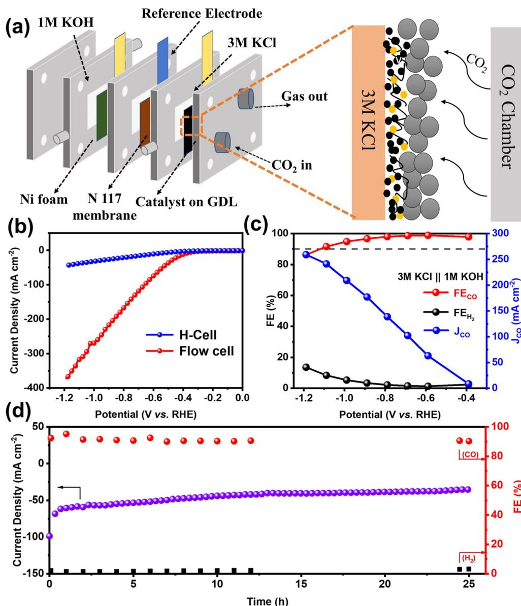
**Fig. 4** (a) Schematic configuration of a flow cell reactor with a GDL loaded with catalyst; (b) LSV curves of NiFe-NC measured in the flow cell; (c)  $FE_{CO}$  and corresponding current densities of NiFe-NC in the flow cell; and (d) stability test for NiFe-NC at  $-0.59$  V vs. RHE with 25 h of continuous electrolysis in the flow cell.
