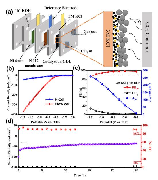
Fig. 4 (a) Schematic configuration of a flow cell reactor with a GDL loaded with catalyst; (b) LSV curves of NiFe-NC measured in the flow cell; (c) FE<sub>CO</sub> and corresponding current densities of NiFe-NC in the flow cell; and (d) stability test for NiFe-NC at -0.59 V vs. RHE with 25 h of continuous electrolysis in the flow cell.
