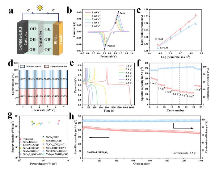
Fig. 7 (a) Schematic illustration of the CoNiMn-LDH//Bi<sub>2</sub>O<sub>3</sub> alkaline battery. (b) CV curves. (c) Plots of log(i) versus log(v). (d) Capacitance contribution. (e) GCD curves. (f) Rate performance. (q) Ragone plots. (h) Cycling performance.
