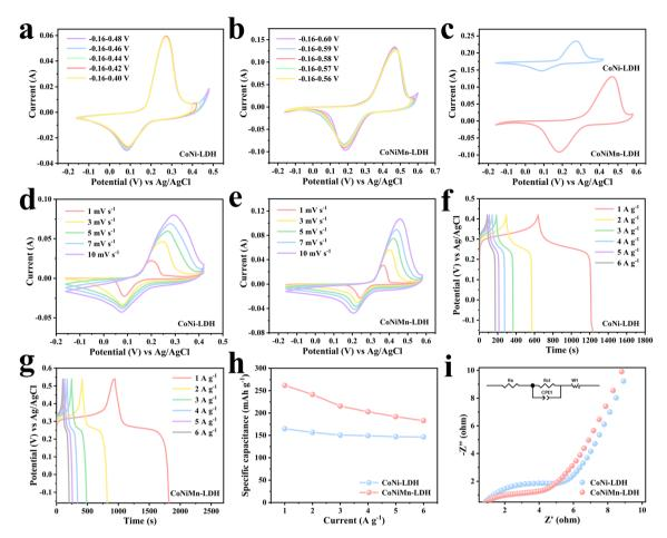
Fig. 4 (a and b) CV curves of CoNi-LDH and CoNiMn-LDH at 10 mV s<sup>-1</sup>. (c) Optimal voltage windows. (d and e) CV curves at different scan rates. (f and g) GCD curves. (h) Specific capacity. (i) Nyquist plots.
