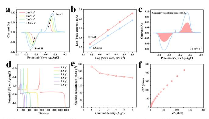
Fig. 6 Electrochemical performance of Bi<sub>2</sub>O<sub>3</sub>. (a) CV curves at different scan rates. (b) Plots of log(i) versus log(v). (c) Capacitive contribution. (d) GCD curves. (e) Specific capacity. (f) Nyquist plots.
