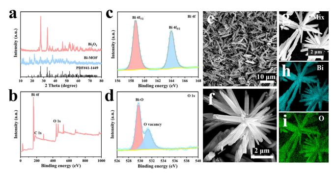
Fig. 5 (a) XRD patterns of Bi-MOF and Bi<sub>2</sub>O<sub>3</sub>. (b) XPS survey of Bi<sub>2</sub>O<sub>3</sub>. (c and d) XPS spectrum of Bi 4f and O 1s of Bi<sub>2</sub>O<sub>3</sub>. (e and f) SEM images of Bi<sub>2</sub>O<sub>3</sub>. (g-i) EDS mapping of Bi<sub>2</sub>O<sub>3</sub>.
