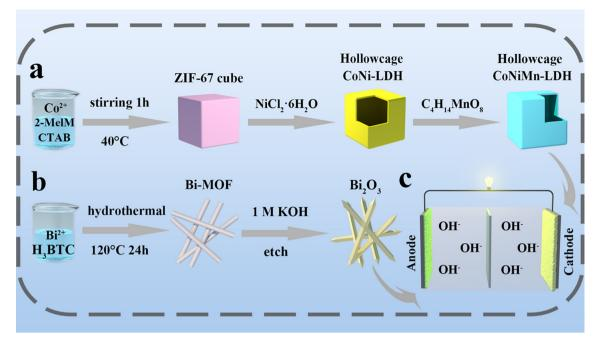
Fig. 1 (a) Schematic diagram of CoNi-LDH and CoNiMn-LDH, (b) Bi<sub>2</sub>O<sub>3</sub>, and the (c) CoNiMn-LDH//Bi<sub>2</sub>O<sub>3</sub> full battery.
