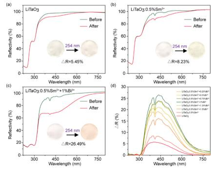
Fig. 2 DRS and color change photos before and after 254 nm light irradiation: (a) LiTaO<sub>3</sub>; (b) LiTaO<sub>3</sub>:0.5 mol% Sm<sup>3+</sup>; (c) LiTaO<sub>3</sub>:0.5 mol% Sm<sup>3+</sup>/ 1 mol%  $\mathrm{Bi}^{3+}$ ; (d) reflectivity different spectra of  $\mathrm{LiTaO_3}$ : 0.5 mol%  $\mathrm{Sm}^{3+}/x$  mol%  $\mathrm{Bi}^{3+}$  (x=0,0.25,0.5,0.75,1,1.25,1.5) powders before and after 254 nm light irradiation.
