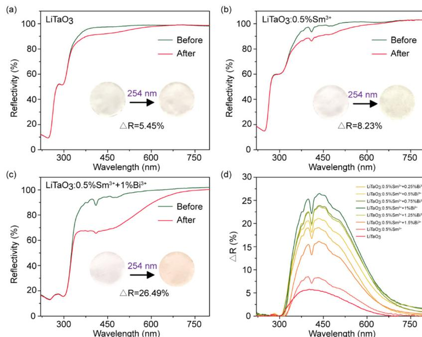
**Fig. 2** DRS and color change photos before and after 254 nm light irradiation: (a)  $\text{LiTaO}_3$ ; (b)  $\text{LiTaO}_3:0.5 \text{ mol\% Sm}^{3+}$ ; (c)  $\text{LiTaO}_3:0.5 \text{ mol\% Sm}^{3+}/1 \text{ mol\% Bi}^{3+}$ ; (d) reflectivity different spectra of  $\text{LiTaO}_3$  and  $\text{LiTaO}_3:0.5 \text{ mol\% Sm}^{3+}/x \text{ mol\% Bi}^{3+}$  ( $x = 0, 0.25, 0.5, 0.75, 1, 1.25, 1.5$ ) powders before and after 254 nm light irradiation.
