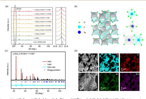
Fig. 1 (a) XRD patterns of the LiTaO<sub>3</sub> and LiTaO<sub>3</sub>:0.5 mol% Sm<sup>3+</sup>/x mol% Bi<sup>3+</sup> (x = 0, 0.25, 0.5, 0.75, 1, 1.25, 1.5); right panel: partial enlargement of the diffraction peak of (012) in the range of 23.6°-23.8°. (b) Crystal structure of the LiTaO<sub>3</sub> host; (c) Rietveld refinement of LiTaO<sub>3</sub>:0.5 mol% Sm<sup>3+</sup>/ 1 mol%  $Bi^{3+}$ ; (d) SEM and elemental EDS mapping of LiTaO<sub>3</sub>:0.5 mol%  $Sm^{3+}/1$  mol%  $Bi^{3+}$ .
