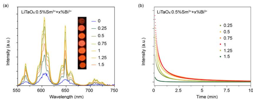
**Fig. 4** (a) PersL spectra of  $\text{LiTaO}_3:0.5 \text{ mol\% Sm}^{3+}/x \text{ mol\% Bi}^{3+}$  ( $x = 0, 0.25, 0.5, 0.75, 1, 1.25, 1.5$ ) powder irradiated at 254 nm for 30 s. Insets: after-glow photos of the corresponding samples; (b) the afterglow decay curves of  $\text{Sm}^{3+}/\text{Bi}^{3+}$  co-doped samples at room temperature after being irradiated with 254 nm light for 30 s.
