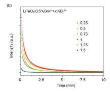
Fig. 4 (a) PersL spectra of LiTaO<sub>3</sub>:0.5 mol% Sm<sup>3+</sup>/x mol% Bi<sup>3+</sup> (x = 0, 0.25, 0.5, 0.75, 1, 1.25, 1.5) powder irradiated at 254 nm for 30 s. Insets: afterglow photos of the corresponding samples; (b) the afterglow decay curves of Sm<sup>3+</sup>/Bi<sup>3+</sup> co-doped samples at room temperature after being irradiated with 254 nm light for 30 s.
