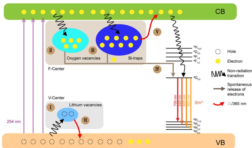
Fig. 6 Schematic diagram of the mechanism of photochromism and PersL processes.
