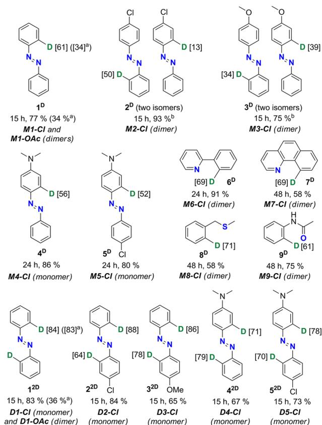
**Chart 1** Products, reaction time and isolated yields of the mechanochemical deuteration of mono- and dipalladated chloride precursors (marked below each product in italic). Percentage of deuteration (average for all magnetically equivalent nuclei) is marked at the site of the D incorporation. <sup>a</sup>Data for the acetate precursors M1-OAc and D1-OAc. <sup>b</sup>Combined yield for two isomeric monodeuterated products.
