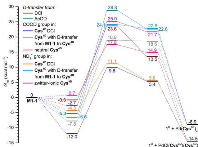
**Fig. 3** D-transfer to **M1-1** from various D-sources. B3LYP-D3/6-311+G\*\*/SDD(Pd)/gas phase free energies reported relative to **M1-1** (in kcal mol<sup>-1</sup>).
