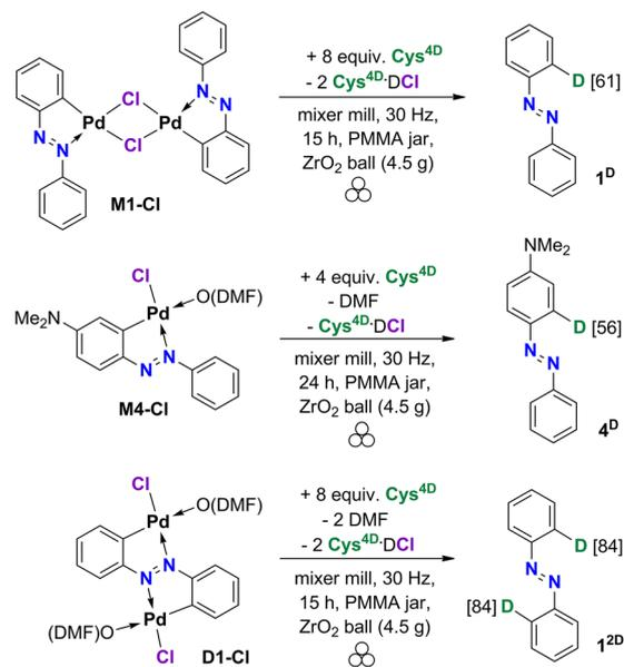
**Scheme 2** Reaction conditions using three characteristic azobenzene complexes.
