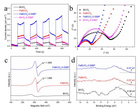
Fig. 7 (a) Photocurrent response and (b) electrochemical impedance spectroscopy (EIS) tests of BiVO<sub>4</sub>, FeBiVO<sub>4</sub>, BiVO<sub>4</sub>-0.05BP and FeBiVO<sub>4</sub>-0.05BP; (c) EPR spectra and (d) XPS valence state spectra of BiVO<sub>4</sub>, FeBiVO<sub>4</sub> and FeBiVO<sub>4</sub>-0.05BP.
