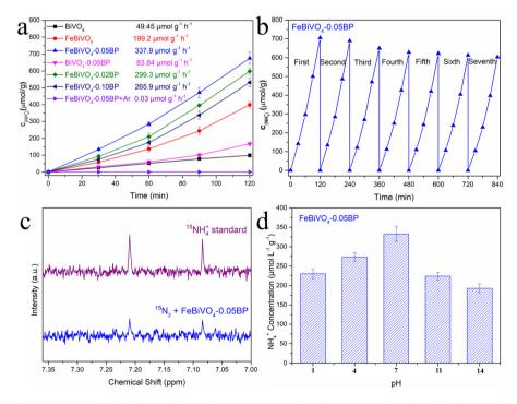
Fig. 5 (a) Photocatalytic N<sub>2</sub> reduction of BiVO<sub>4</sub>, FeBiVO<sub>4</sub>-0.05BP, FeBiVO<sub>4</sub>-0.05BP, FeBiVO<sub>4</sub>-0.02BP and FeBiVO<sub>4</sub>-0.10BP under visible light irradiation. (b) Stability test for the nitrogen reduction of the FeBiVO<sub>4</sub>-0.05BP photocatalyst. (c) <sup>1</sup>H NMR spectra qualitative isotope labeling test of  $FeBiVO_4$ -0.05BP. (d) The  $NH_4^+$  yield of the  $FeBiVO_4$ -0.05BP sample under different pH conditions after 2 h.
