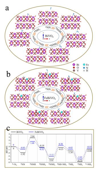
Fig. 6 Optimized structures of reaction intermediates in a distal mechanism: (a) BiVO<sub>4</sub> and (b) FeBiVO<sub>4</sub>; (c) Gibbs free energy profiles of nitrogen reduction over BiVO<sub>4</sub> and FeBiVO<sub>4</sub> catalysts by a distal mechanism.
