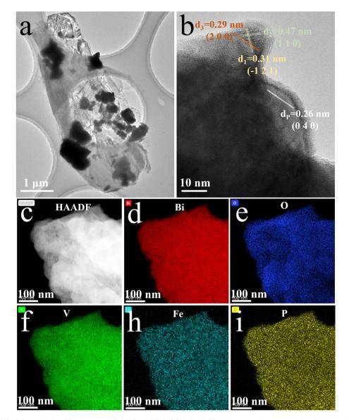
Fig. 3 (a) TEM and (b) High-resolution TEM images of FeBiVO<sub>4</sub>-0.05BP; (c) HADDF-STEM image and corresponding EDS mapping: (d) Bi, (e) O, (f) V, (h) Fe, (i) P.
