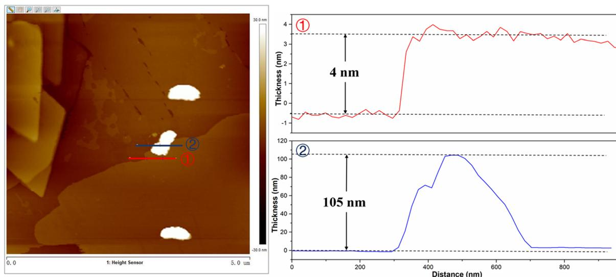
Fig. 2 AFM images of FeBiVO<sub>4</sub>-0.05BP (left) and the corresponding thickness distribution (right).
