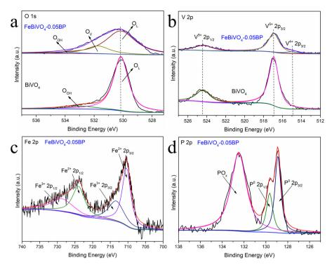
Fig. 4 High-resolution XPS of (a) O 1s and (b) V 2p for BiVO<sub>4</sub> and FeBiVO<sub>4</sub>-0.05BP, high-resolution XPS of (c) Fe 2p and (d) P 2p for FeBiVO<sub>4</sub>-0.05BP.
