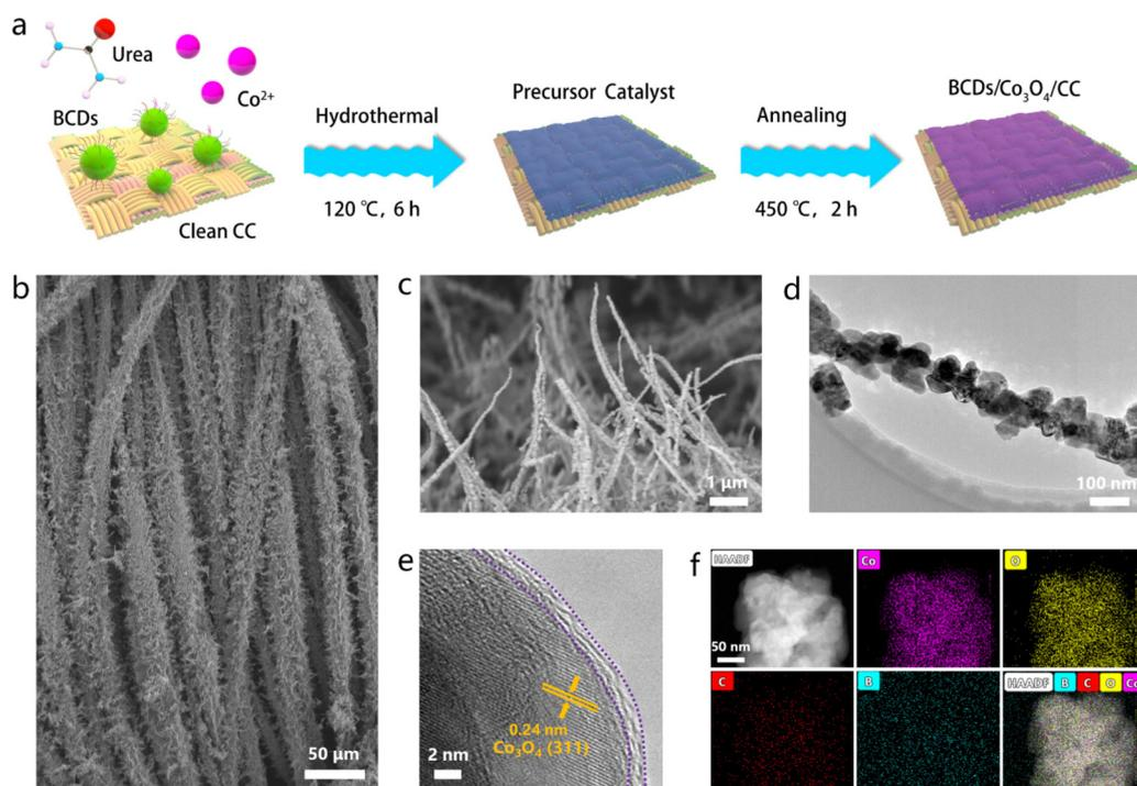
**Fig. 1** Synthesis and characterization of BCDs/Co<sub>3</sub>O<sub>4</sub>/CC. (a) Schematic illustration of the synthesis of BCDs/Co<sub>3</sub>O<sub>4</sub>/CC. (b) SEM image of the precursor catalyst. (c–e) SEM, TEM and HRTEM images of BCDs/Co<sub>3</sub>O<sub>4</sub>/CC. (f) Element mapping images of BCDs/Co<sub>3</sub>O<sub>4</sub>/CC.
