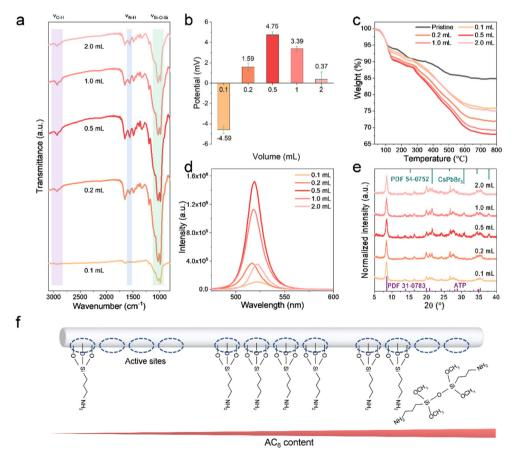
Fig. 4 (a) FTIR spectra, (b) zeta potentials and (c) TG curves of ATP with varying APTMS modification contents. (d) PL spectra and (e) the corresponding XRD patterns of the ATP-A<sub>C6</sub>@CsPbBr<sub>3</sub> nanocomposite with different APTMS modification contents. (f) Schematic diagram of the relationship between reactive sites and APTMS content.
