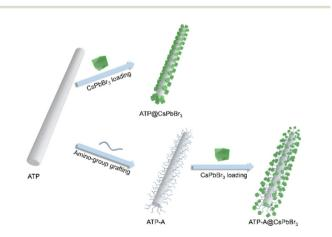
Fig. 1 Schematic diagram of the construction of ATP@CsPbBr3 and ATP-A@CsPbBr3 nanocomposites.
