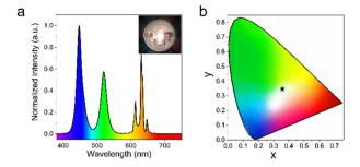
Fig. 6 (a) Emission spectra of a white LED fabricated by depositing green ATP-A<sub>C6</sub>@CsPbBr<sub>3</sub> nanocomposite and the commercial red phosphor  $K_2SiF_6$ :  $Mn^{4+}$  on a blue InGaN chip under a current of 100 mA. The inset shows a photograph of the operating white LED. (b) CIE color diagram of the white LED device.
