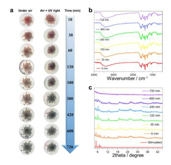
Fig. 4 Color-change map of cluster 1 at different time points under the conditions of air and UV light exposure (a). FTIR spectra and PXRD patterns of cluster 1 at different time points in air (b and c).
