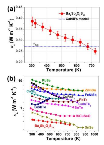
Fig. 4 (a) Lattice thermal conductivity  $(k_1)$  as a function of temperature for  $Ba_6Sb_6O_2S_{13}$  (the dashed line represents the minimum  $k_L$  value calculated within the Cahill model) and (b) comparison of  $k_L$  with other reported state-of-the-art thermoelectric materials.
