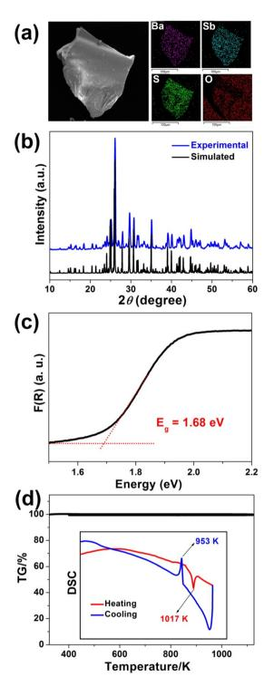
Fig. 3 Experimental characterization of Ba<sub>6</sub>Sb<sub>6</sub>O<sub>2</sub>S<sub>13</sub>: (a) the SEM image and the corresponding elemental mapping analysis; (b) experimental (blue) and simulated (black) PXRD patterns; (c) the solid-state diffusereflectance spectrum; (d) TG diagram (inset: DSC cyclic curves).
