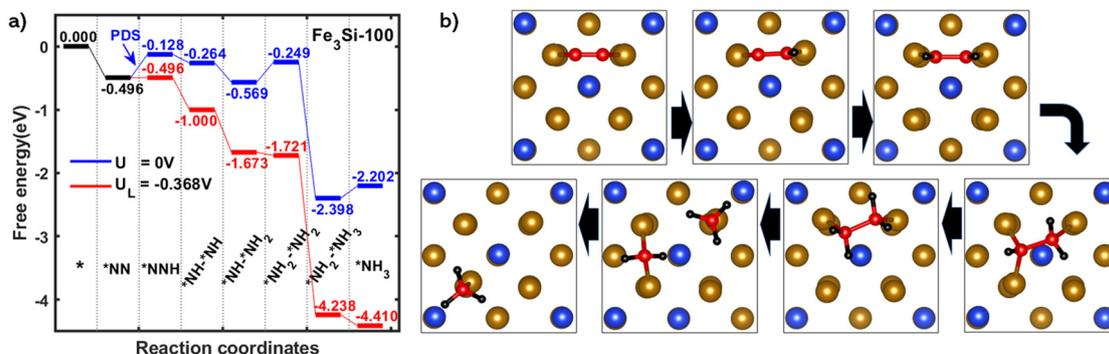
**Fig. 3** (a): Free energy evolution of the e-N<sub>2</sub>RR on the  $Fe_3Si(100)$  surface with PDS identified as the first protonation step. (b): Top views of adsorption configurations of all intermediates during the enzymatic pathway. Color map: bronze – Fe; blue – Si; red – N; and black – H.
