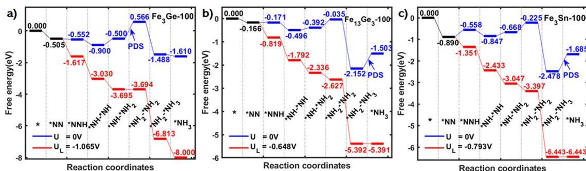
Fig. 4 Free energy diagrams of electrochemical nitrogen reduction on (a) Fe<sub>3</sub>Ge, (b) Fe<sub>13</sub>Ge<sub>3</sub> and (c) Fe<sub>3</sub>Sn, respectively. The best results among group-IV elements follow the sequence “Si > Ge > Sn”.
