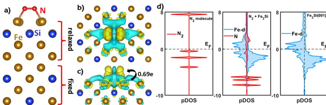
**Fig. 2** (a): Horizontal mode of  $N_2$  adsorption on the  $Fe_3Si(100)$  surface. (b) and (c): Top and side views of the charge density difference plot of  $N_2$  adsorption on the  $Fe_3Si(100)$  surface. Yellow indicates charge accumulation and cyan represents charge depletion. The isosurface value is set to be  $0.001 e \text{ Bohr}^{-3}$ . (d): Projected density of states (PDOS) of isolated  $N_2$ ,  $N_2$  adsorbed  $Fe_3Si$ , and  $Fe_3Si$ .
