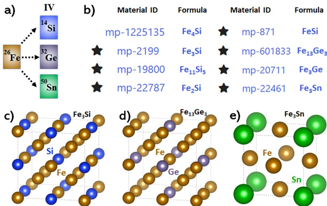
**Fig. 1** (a): Fe-group-IVA binary alloys studied in this work. (b): Eight candidates of Fe-group-IVA binary alloys with their IDs and formulas from the Materials Project database.<sup>54</sup> (c–e): Conventional cells of some typical atomic structures among all studied candidates.
