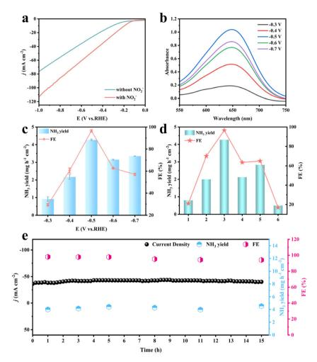
Fig. 3 (a) LSV curves of  $Co_3O_4/NiFe$  LDH-40 in 0.1 M NaOH with/without 0.1 M  $NO_2^-$ . (b) UV-vis spectra, (c) NH<sub>3</sub> yields and FEs of  $Co_3O_4/NiFe$  LDH-40 from -0.3 to -0.7 V. (d) NH<sub>3</sub> yields and FEs belonging to 1. NiFe LDH/NF, 2.  $Co_3O_4/NiF$ , 3.  $Co_3O_4/NiFe$  LDH-40, 4.  $Co_3O_4/NiFe$  LDH-20, 5.  $Co_3O_4/NiFe$  LDH-60, and 6. NF. (e) Long-term experiment of electrochemical nitrate reduction at -0.5 V and the associated NH<sub>3</sub> yields and FEs.
