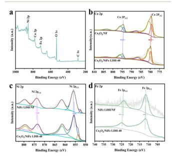
Fig. 2 (a) XPS survey spectrum of Co<sub>3</sub>O<sub>4</sub>/NiFe LDH-40. (b) Co 2p, (c) Ni 2p and (d) Fe 2p XPS spectra of related materials.
