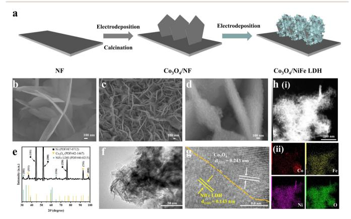
Fig. 1 (a) Illustration of the Co<sub>3</sub>O<sub>4</sub>/NiFe LDH synthesis. SEM images of (b) Co<sub>3</sub>O<sub>4</sub>/NF, (c) NiFe LDH/NF and (d) Co<sub>3</sub>O<sub>4</sub>/NiFe LDH-40. (e) XRD pattern of Co<sub>3</sub>O<sub>4</sub>/NiFe LDH-40. (f) TEM and (g) HRTEM images of Co<sub>3</sub>O<sub>4</sub>/NiFe LDH-40. (h) TEM and the corresponding elemental mapping images of Co<sub>3</sub>O<sub>4</sub>/NiFe LDH-40.
