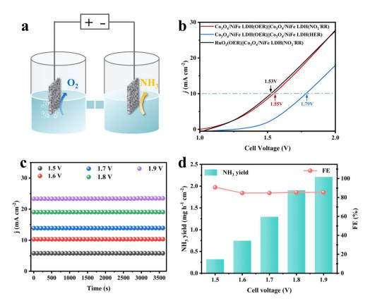
Fig. 5 (a) Illustration of the two-electrode OER $|NO_2$ -RR electrolyzer. (b) LSV curves of relevant two-electrode systems. (c) Chronoamperometry curves, (d) NH<sub>3</sub> yield rate and FE of Co<sub>3</sub>O<sub>4</sub>/NiFe LDH-40 in the OER $|NO_2$ -RR system at various applied cell voltages.
