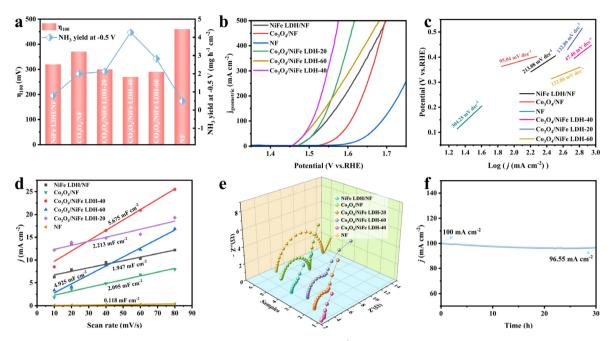
Fig. 4 (a) The comparison of  $NH_3$  yield at -0.5 V and overpotential at 100 mA cm<sup>-2</sup> of different materials. (b) OER polarization curves based on geometric area, (c) OER Tafel curves, (d)  $C_{dl}$  values and (e) Nyquist plots of different electrocatalysts. (f) Chronoamperometric measurements of  $Co_3O_4/$ NiFe LDH-40.
